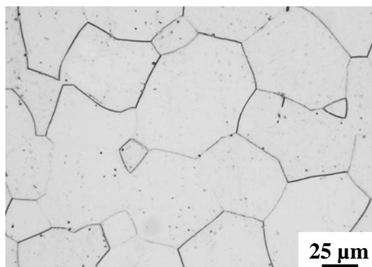
Fig. 1. Optical microstructure of the Ti-15-3 base material.
