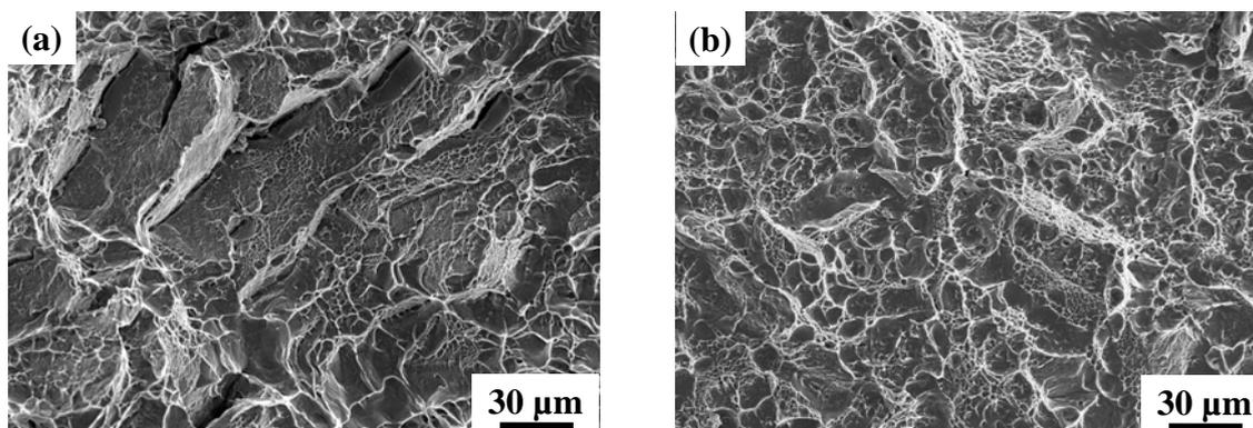
Fig. 4. SEM fractographs of the (a) D426 and (b) D538 specimens
