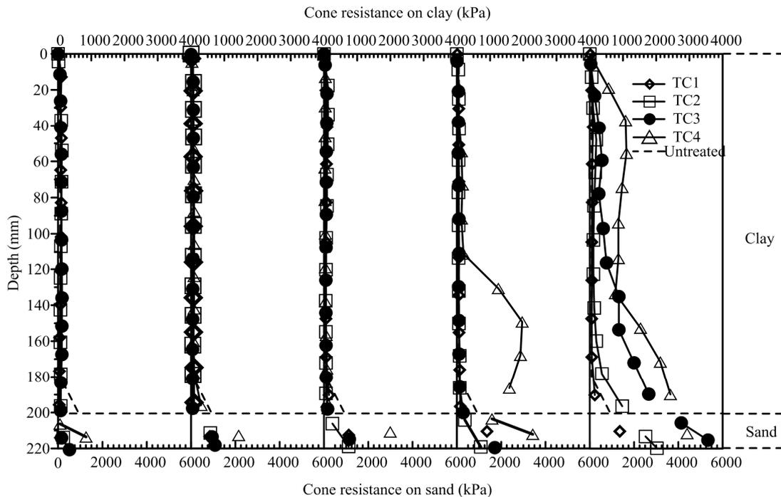
Fig. 4 Profiles of cone resistance for different treatment times with injection of calcium chloride.
