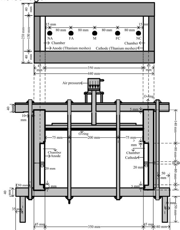
Fig. 1 Schematic configuration of the electroosmotic cell (top view and side view).
