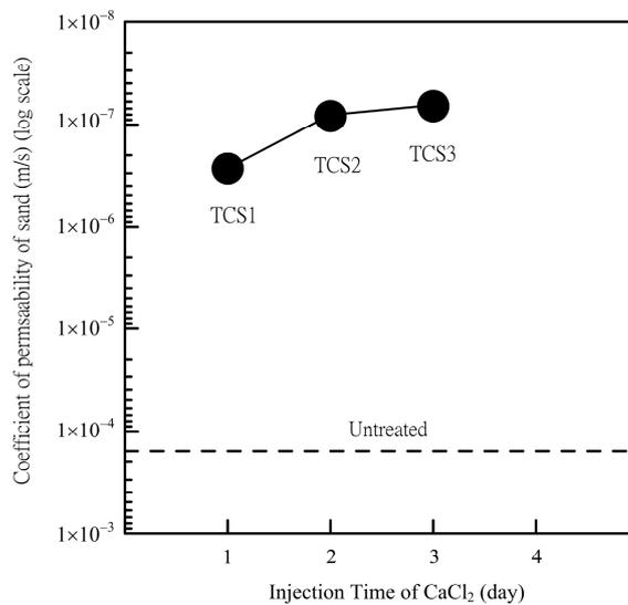
Fig. 3 Effect of different treatment times with injection of calcium chloride, followed by injection of the sodium silicate solution, on the permeability coefficient of sand.
