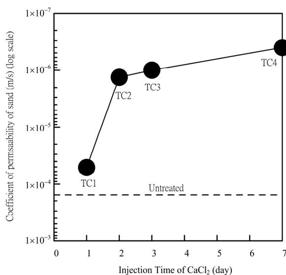
Fig. 2 Effect of different treatment times with injection of calcium chloride on the permeability coefficient of sand.
