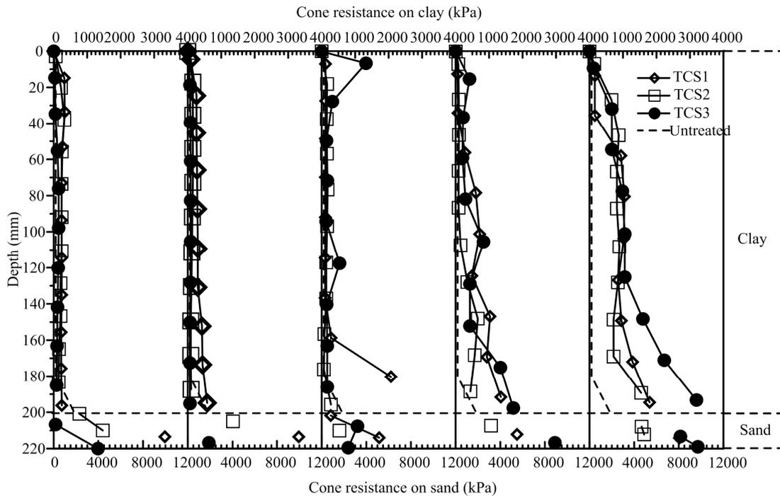
Fig. 5 Profiles of cone resistance for different treatment times with injection of calcium chloride, followed by injection of the sodium silicate solution.
