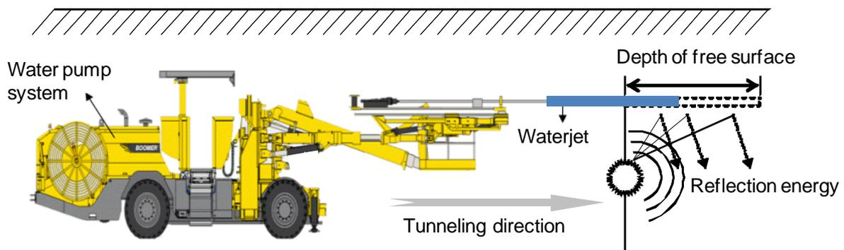
Fig. 1. Concept of rock excavation method using abrasive waterjet system
