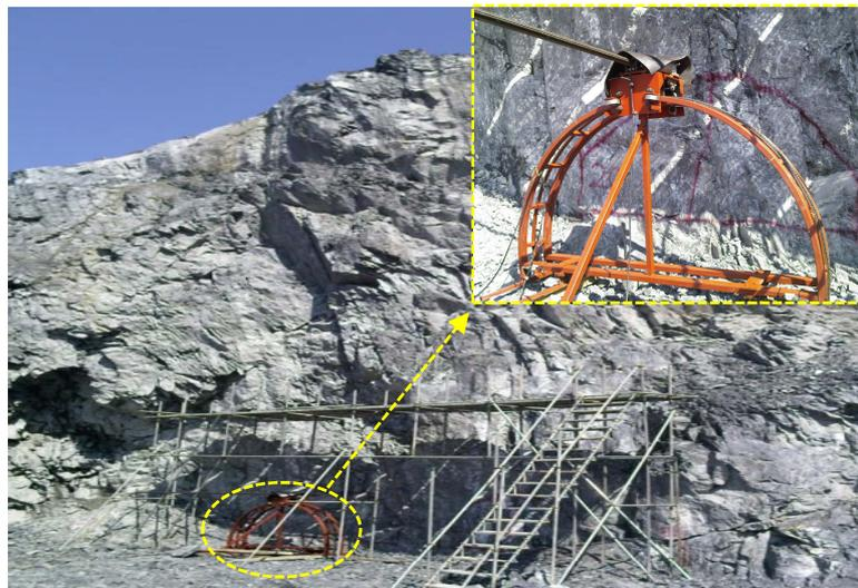
Fig. 4. Abrasive waterjet system setup
