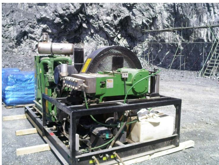
Fig. 3. A plunger type pump
