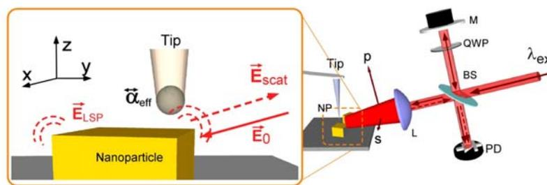
**Fig. 2.** The operation principle of the sSNOM (left) and the detailed detection schemes (right).  $E_{scat}$  = scattered field,  $E_0$  = incident field, and  $E_{LSP}$  = localized plasmonic field,  $\alpha_{eff}$  = effective polarizability of the tip, M = mirror, QWP = quarter-wave plate, BS = 50/50 beam splitter, NP = nanoparticle, and PD = photodiode.
