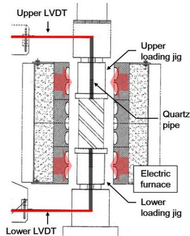
Fig. 2 Experimental apparatus used in this study
