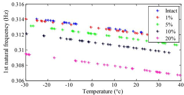
Fig. 7 Temperature versus 1st natural frequency
