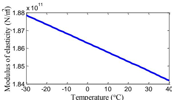
Fig. 2 Temperature versus modulus of elasticity
