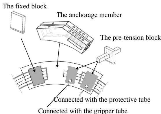
Fig. 4 Detailed diagram of the FBG hoop-strain sensor
