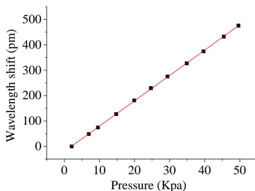
Fig. 6 Calibration of PVC
