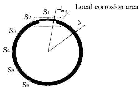
Fig. 3 Diagram of local corrosion and strain measuring point
