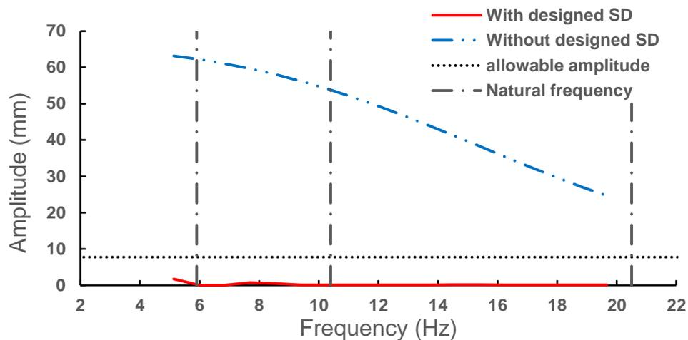
Fig. 2 Amplitudes of the hanger vibration with designed SD
