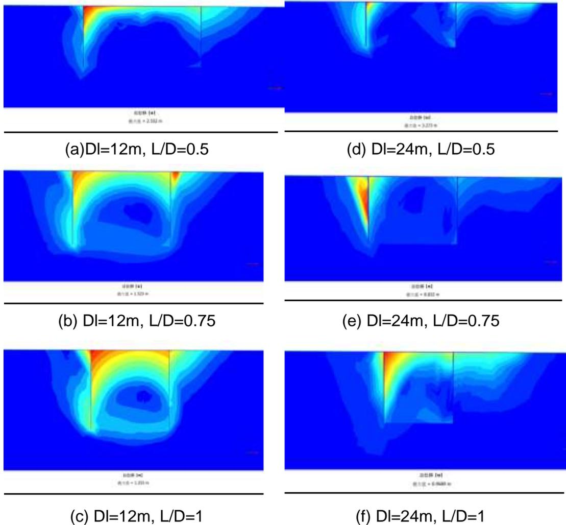
Fig. 7 In comparison to the displacement of the composite suction foundation upper lid diameter DI=12m,24m with different bucket L/D when load eccentricity  $h=70\text{m}$  in dense sand
