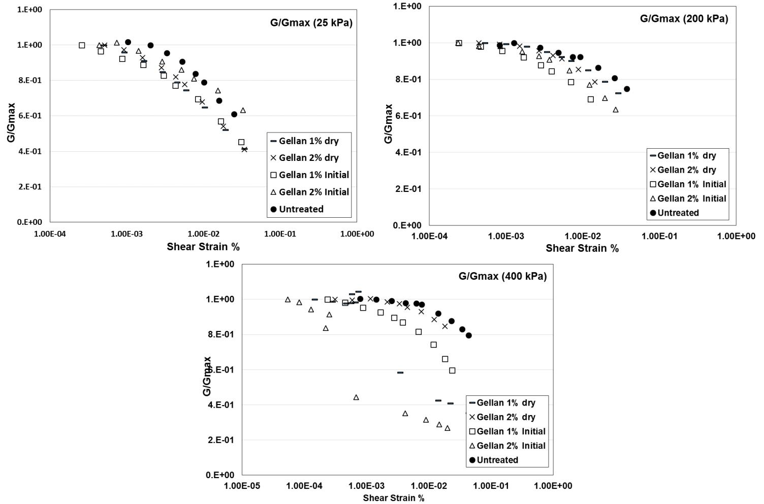
Fig. 3  $G/G_{\max}$  curves of untreated and gellan treated soils
