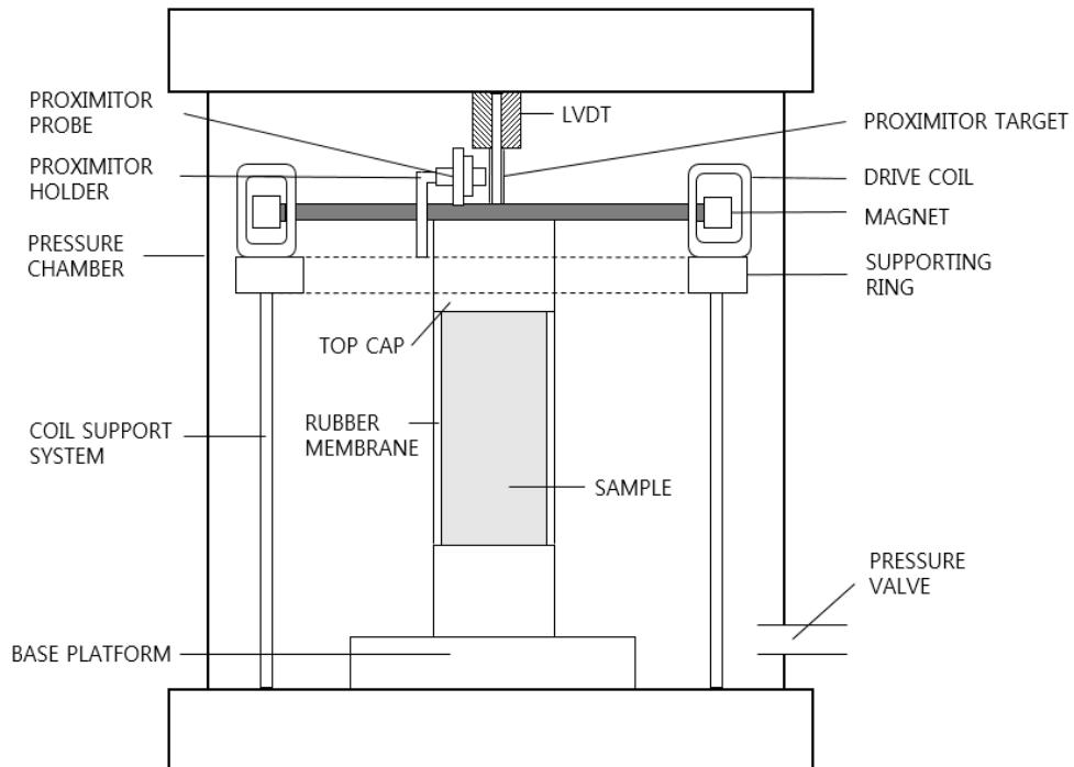
Fig. 2 Resonant column testing apparatus
