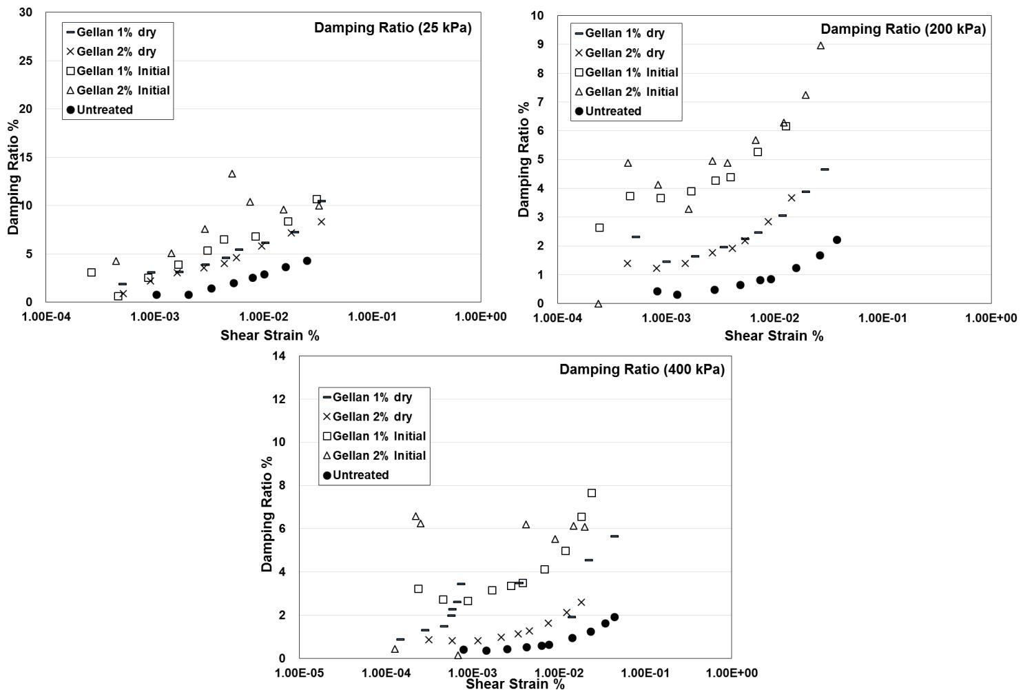
Fig. 4 Damping ratios of gellan treated and untreated sands
