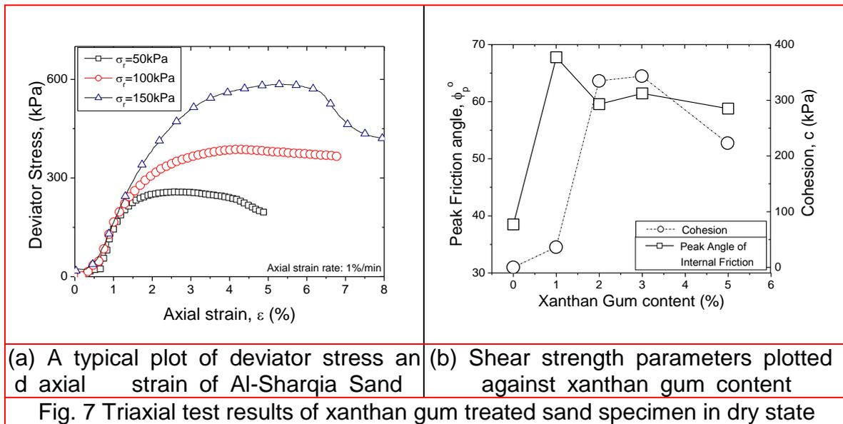
(a) A typical plot of deviator stress and axial strain of Al-Sharqia Sand (b) Shear strength parameters plotted against xanthan gum content
