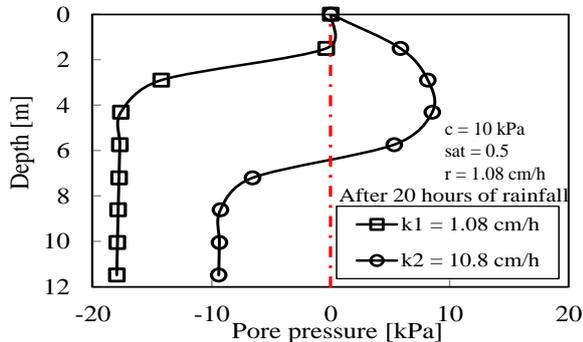
Figure 3. Change in pore pressure after 20 hours of 1.08 cm/h rainfall
