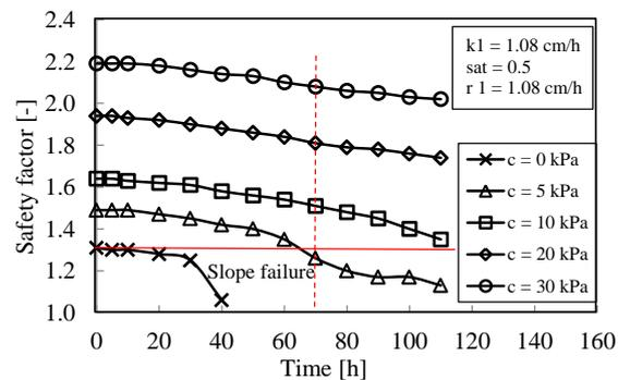
Figure 9. Effects of effective cohesion on safety factor
