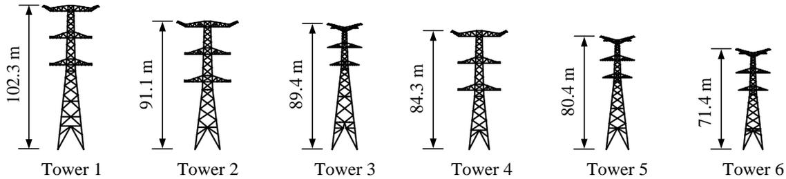
Fig. 4 Transmission towers with cantilevered cross-arms used in the statistical analysis
