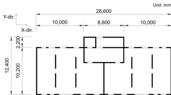
Fig.1 Structural plan of the case study building
