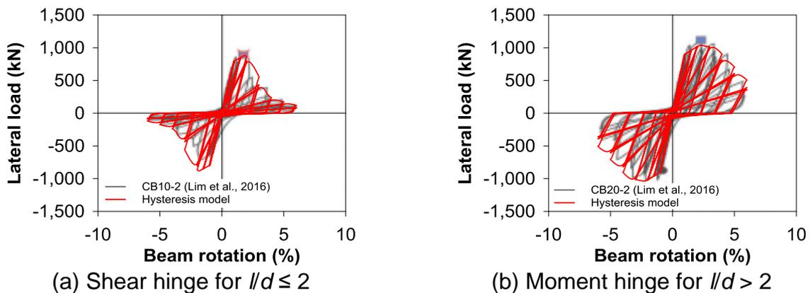
Fig.2 Hysteresis modeling of coupling beams
