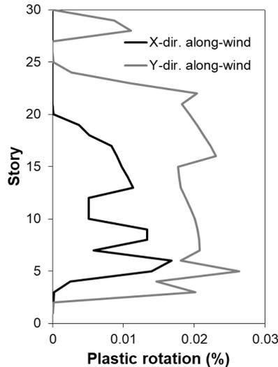
Fig. 4 Plastic rotation of coupling beams
