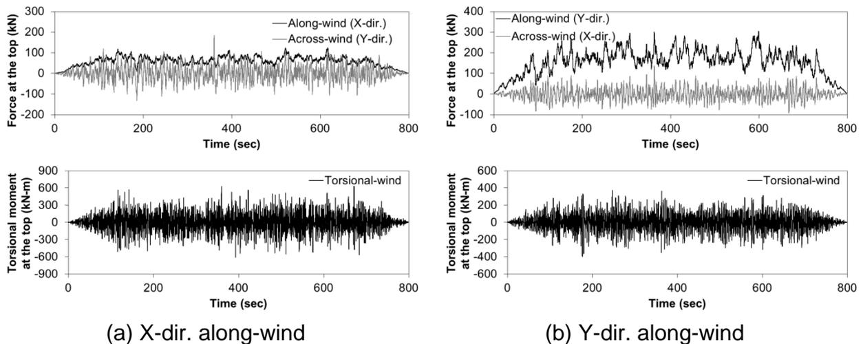
Fig. 3 Time history wind loads generated from PSD functions
