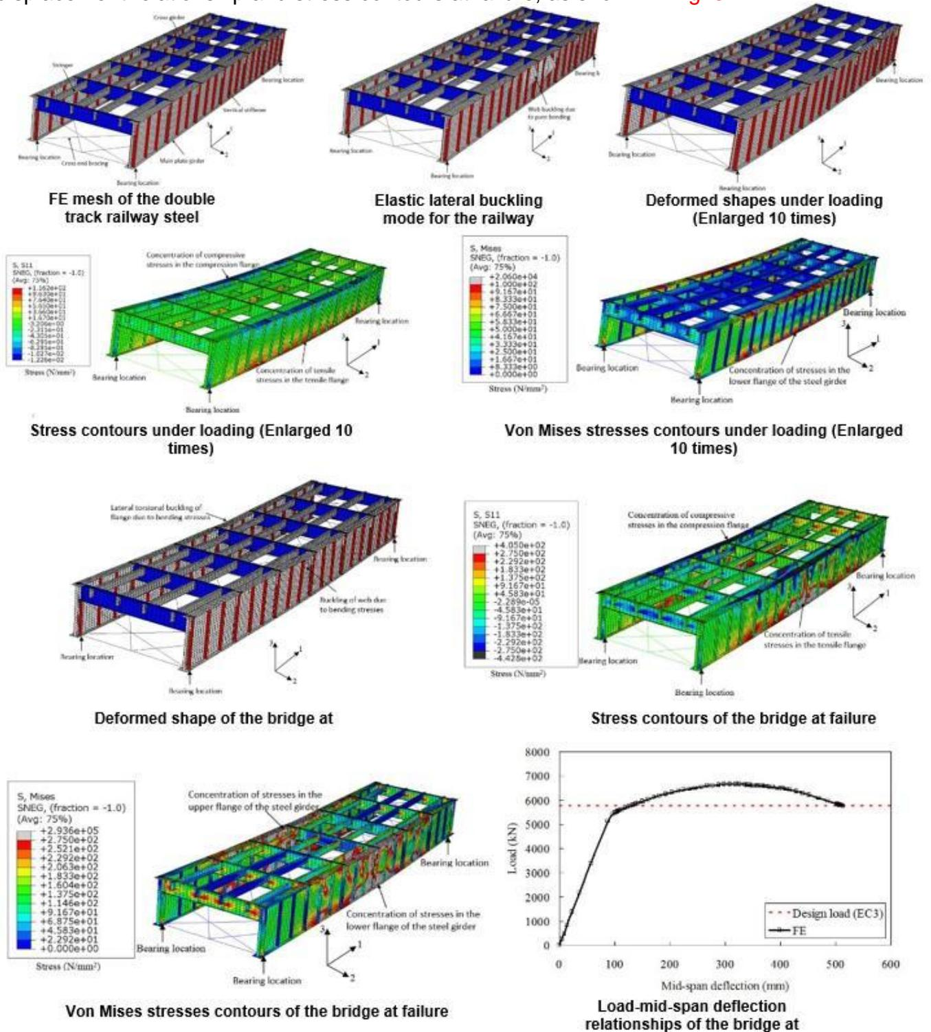
Fig. 3 FE modelling results of the double track railway bridge components detailed in (Ellobody 2014)
