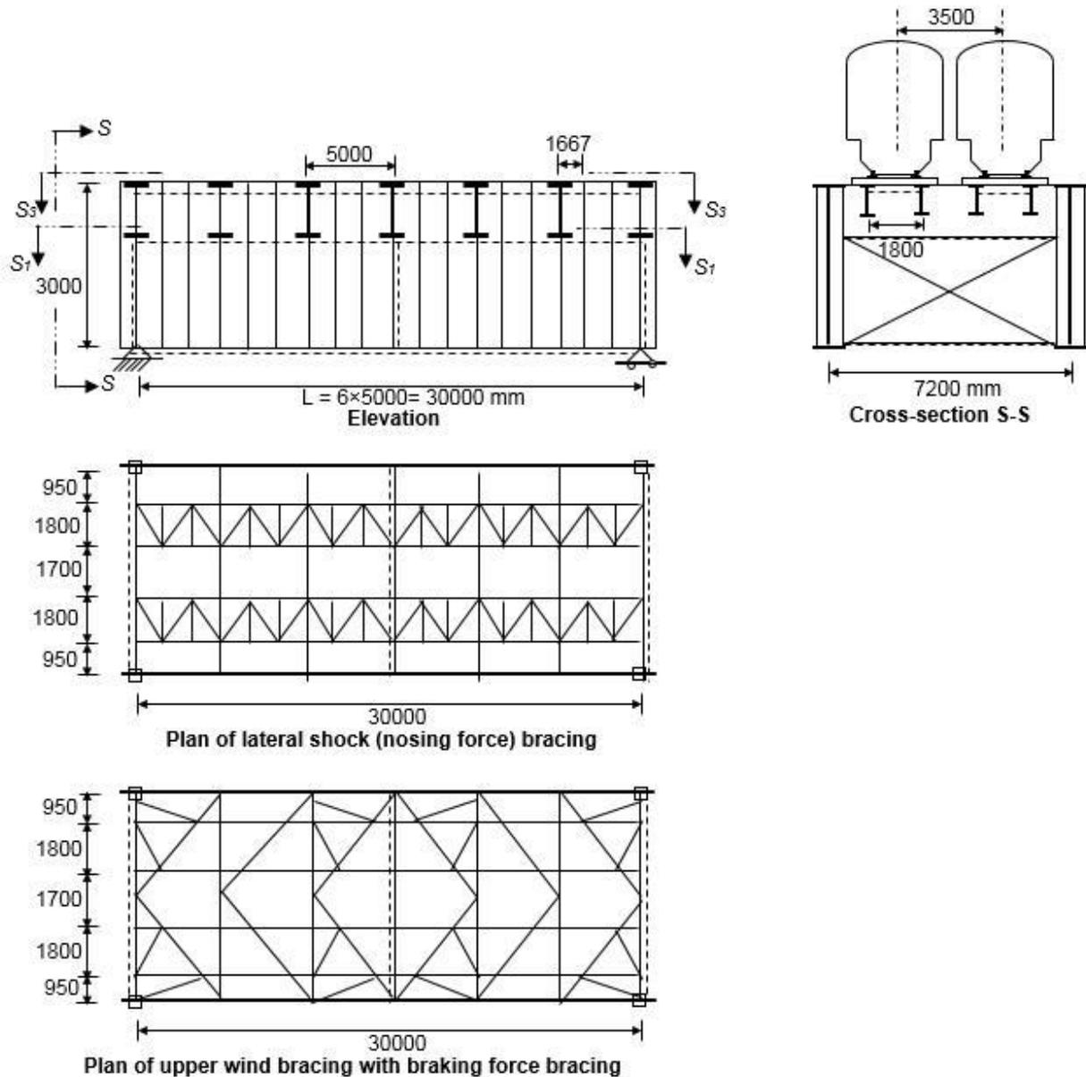
Fig. 1(b) General layout of the double track plate girder railway steel bridge detailed in (Ellobody 2014)
