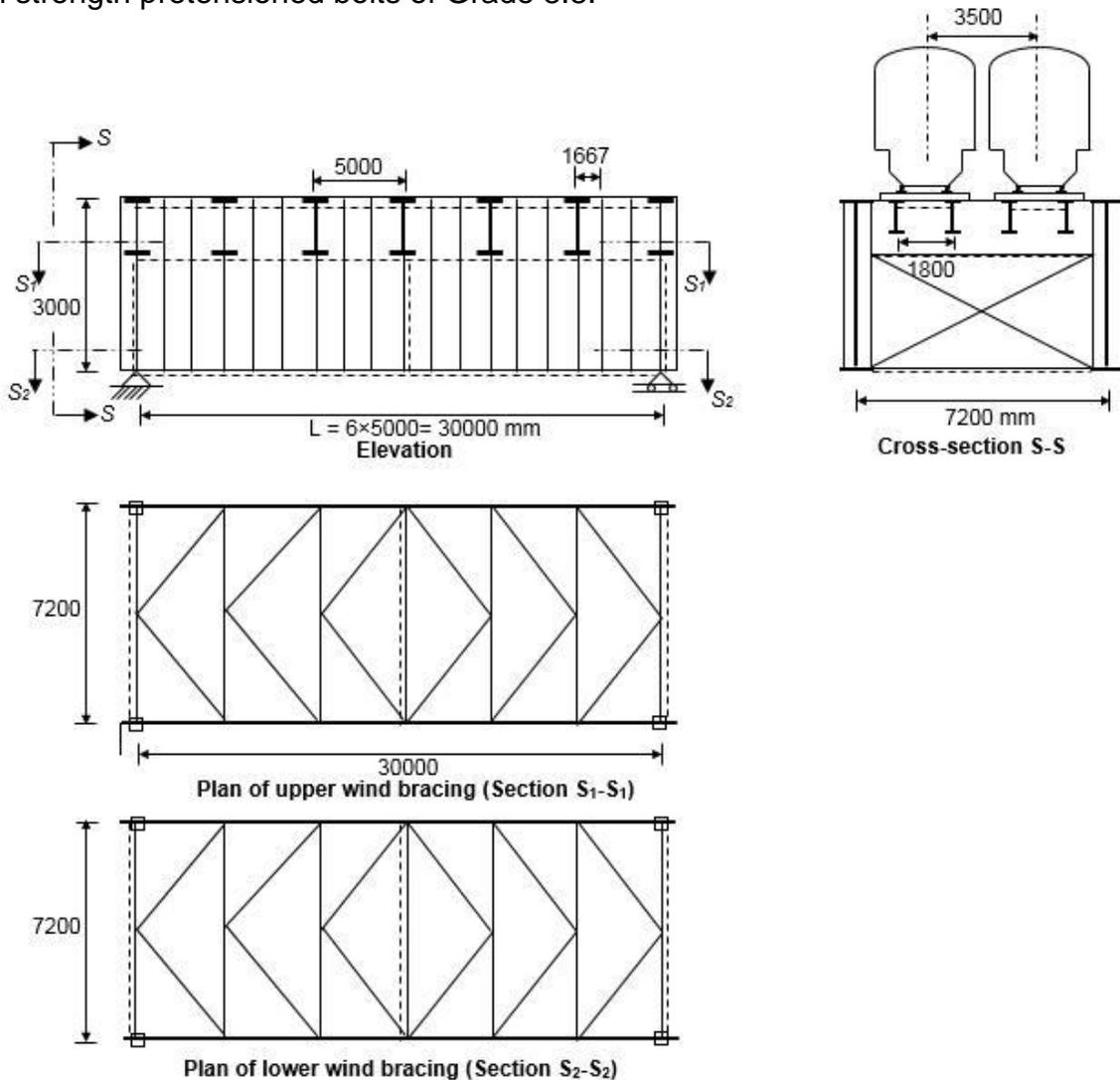
**Fig. 1(a)** General layout of a double track open-timber floor plate girder deck railway steel bridge detailed by the author in (Ellobody 2014)
