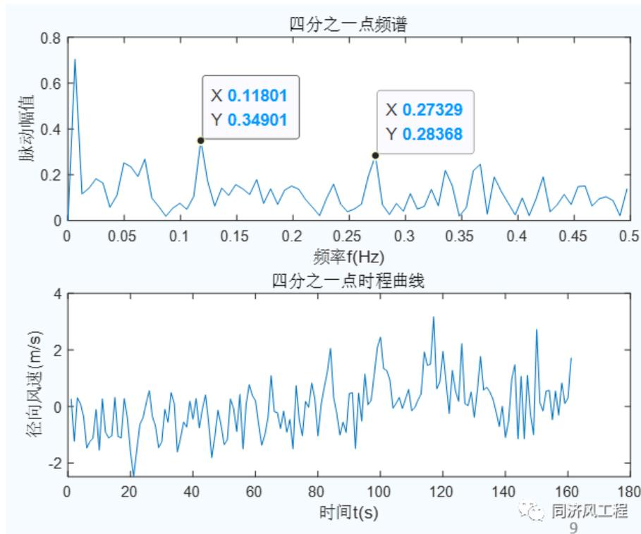
Fig.6 Obvious vortex shedding in the wake flow of the original main girder section of Humen Bridge (after removing the water horse) (8 m/s, 0.23 Hz, 12 cm)
