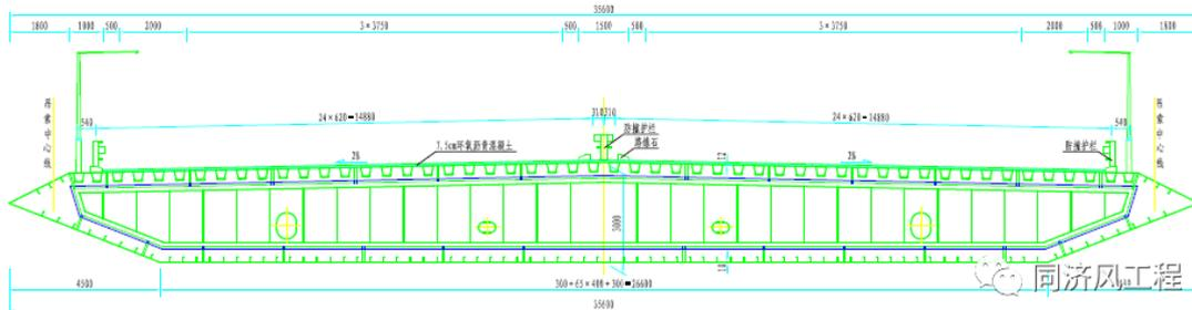
Fig.2 Standard cross-sectional view of stiffening girder of Humen Bridge (Unit: mm)
