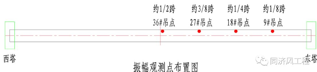
Fig.5 Hangers' number and main amplitude observation points of Humen Bridge
