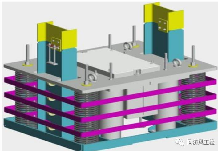
Fig.10 Schematic diagram of TMD damper
