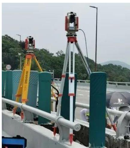
Fig.3 Displacement measurement by video imaging technique
