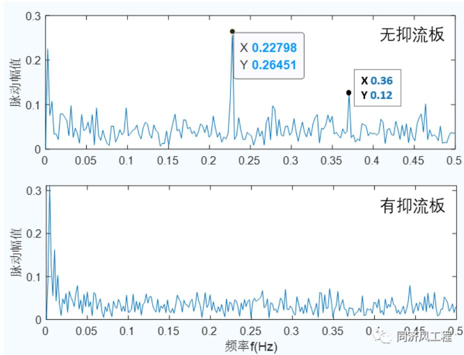
Fig.8 Wake flow vortex breaking effect of spoiler based on comparison of spatial fluctuation velocity spectrum measured by lidar (above without spoilers and below with spoilers)
