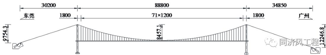
Fig.1 Schematic diagram of structural layout of Humen Bridge (Unit: cm)
