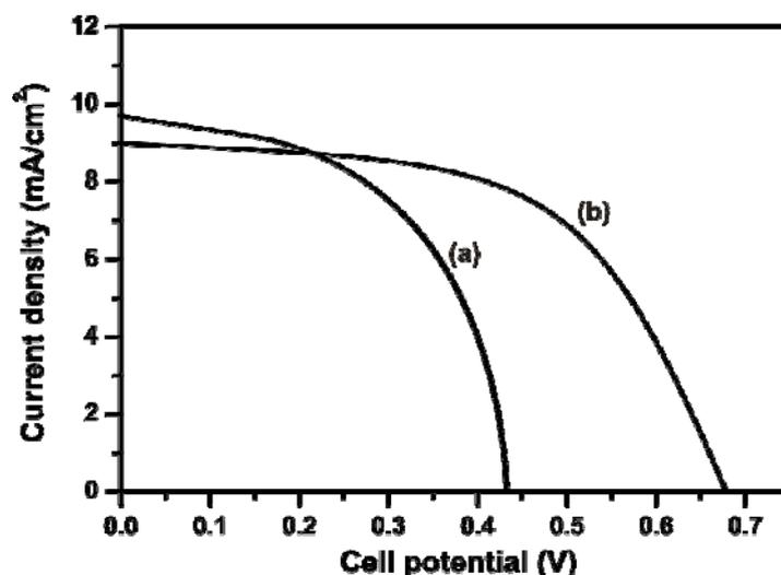
Fig. 4  $I$ - $V$  diagram of (a) dye coated  $\text{WO}_3$ - $\text{TiO}_2$  and (b) dye coated  $\text{CeO}_2$ - $\text{TiO}_2$  photoelectrodes
