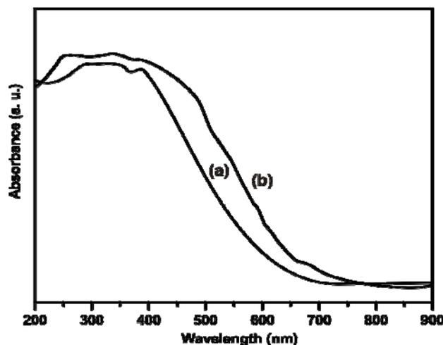
Fig. 3 UV diagram of (a) dye coated  $\text{WO}_3\text{-TiO}_2$  and (b) dye coated  $\text{CeO}_2\text{-TiO}_2$  photoelectrodes
