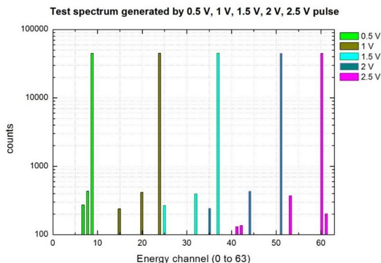
Fig. 2 Test spectrum generated by test pulse
