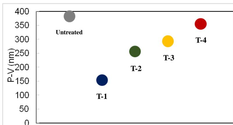
Fig. 6 The relationship between colorization and roughness size (P-V) of Ti surface.
