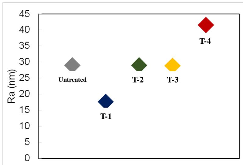
Fig. 5 The relationship between colorization and roughness value (Ra) of Ti surface.
