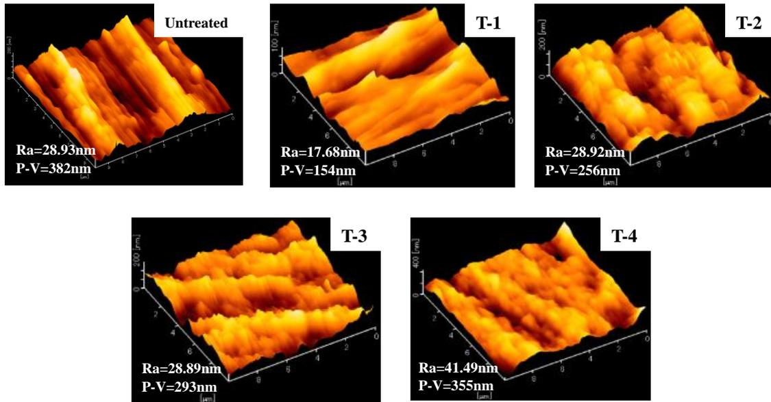
Fig. 4 AFM images of various samples.
