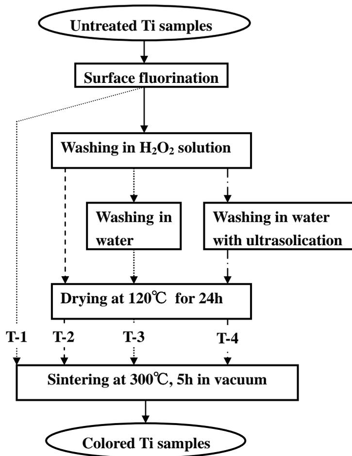
Fig. 1 Flow diagram for coloration of Ti samples
