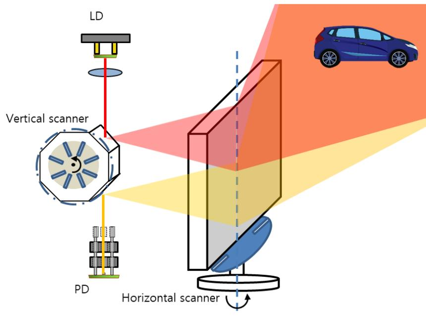
Fig. 4 3D LiDAR configurations using polygon scanner for wide angle scanning
