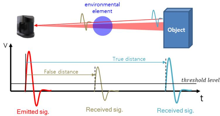
Fig. 1 The measurement error due to environmental effects
