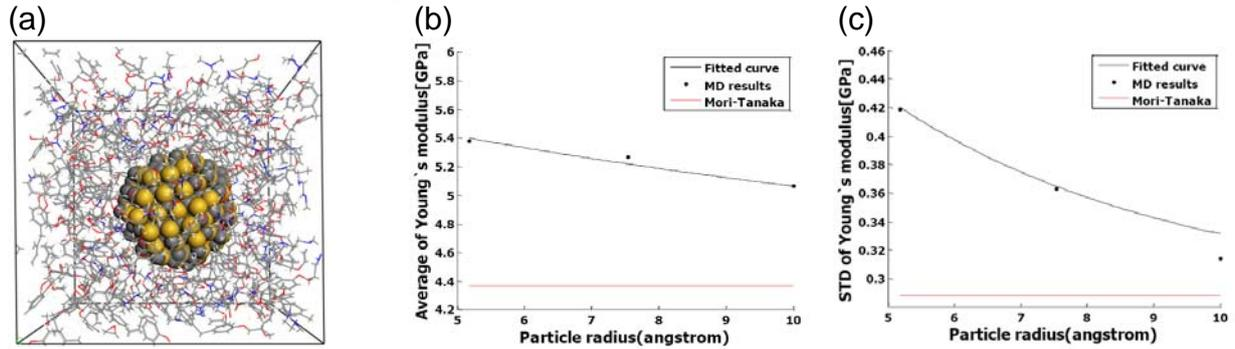
Fig. 1 Quantified MD model uncertainty about various radii: (a) molecular structure, (b) average, and (c) standard deviation.
