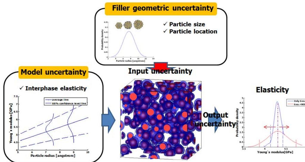
Fig. 3 Integrated multiscale analysis framework merging filler geometric uncertainty with MD model inherent uncertainty
