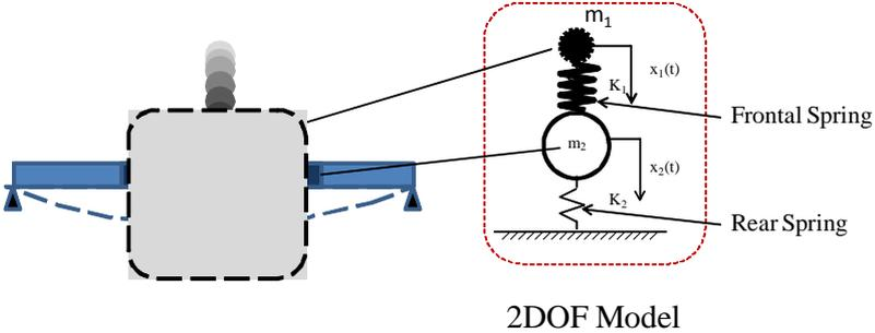
(a) Spring connected lumped masses representing impactor and beam
