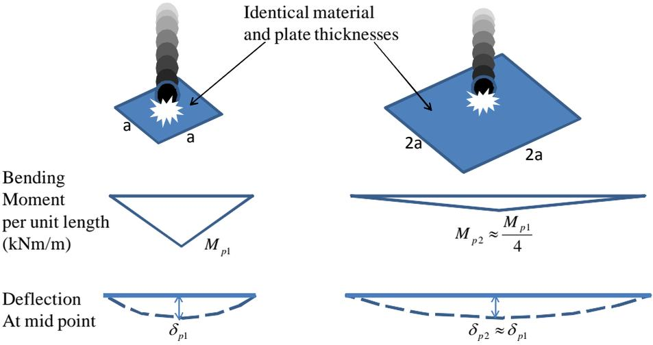
Fig. 3 Scaling relationships for quasi-static impact actions on plates
