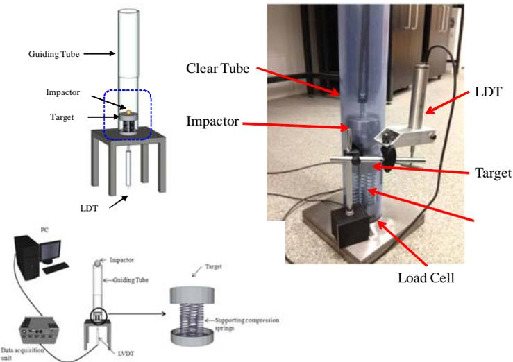
Fig. 5 Custom made tubular device for measuring impact forces
