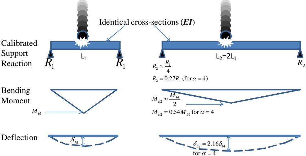
Fig. 2 Scaling relationships for quasi-static impact actions on beams
