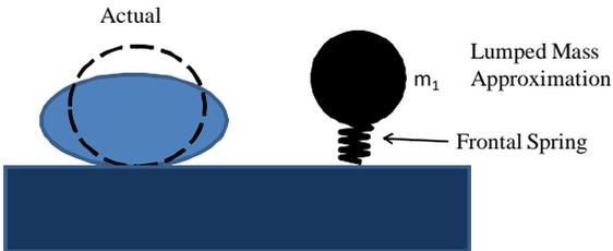
(b) Frontal spring representing deformation behaviour of debris impactor
