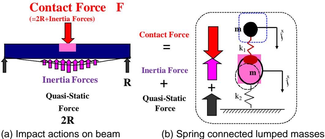
Fig. 1 Contact force versus quasi-static actions
