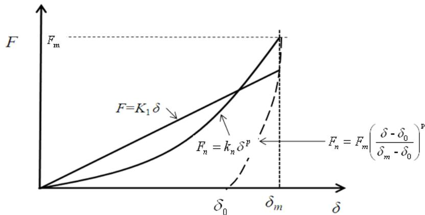
(a) Non-linear inelastic compressive stiffness model of frontal spring
