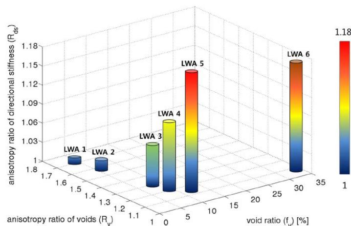
Fig. 1. Correlation between the void ratio, anisotropy ratio of voids, and anisotropy of directional stiffness (Note:  $R_v = \max \bar{P}_{vv} / \min \bar{P}_{vv}$ ,  $R_{ds} = \max(\text{directional stiffness}) / \min(\text{directional stiffness})$ )
