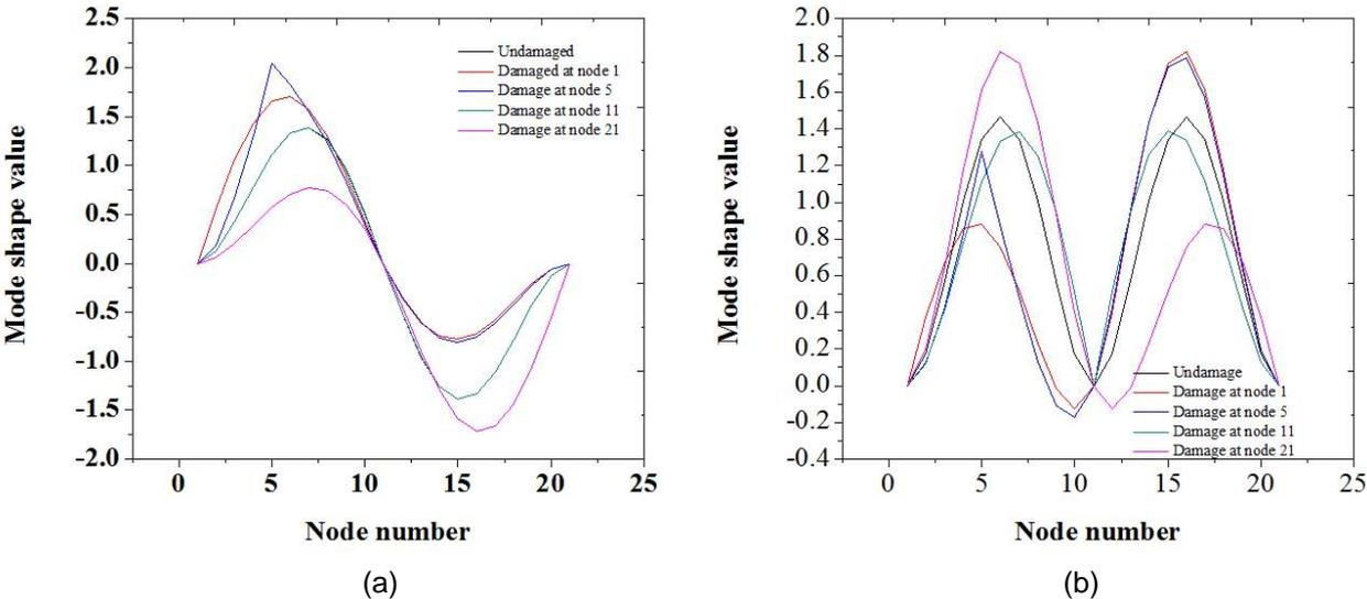
Fig. 2 (a) 1<sup>st</sup> mode shape; (b) 2<sup>nd</sup> mode shape of the continuous beam for undamaged and different damage locations
