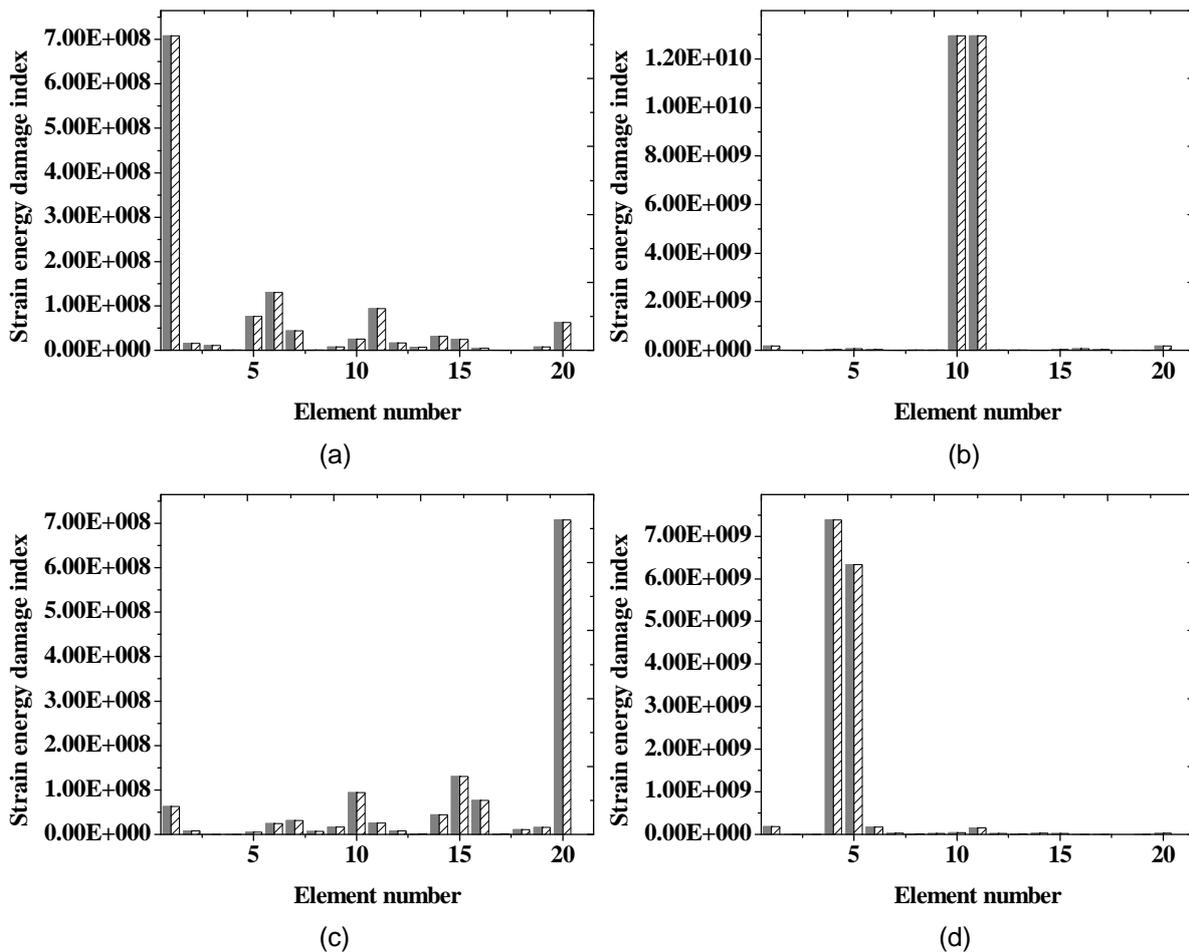
Fig. 4 Modal strain energy damage index ( without noise, with 80db noise): (a) For damage at node 1, (b) For damage at node 11, (c) For damage at node 21, (d) For damage node 5
