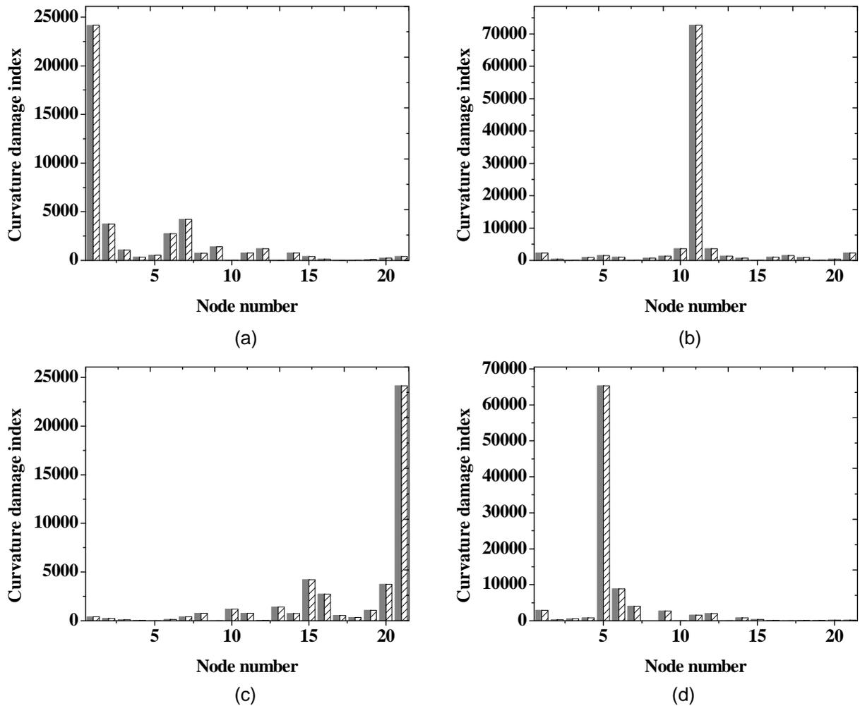
Fig. 3 Curvature damage index (without noise, with 80db noise): (a) For damage at node 1, (b) For damage at node 11, (c) For damage at node 21, (d) For damage at node 5
