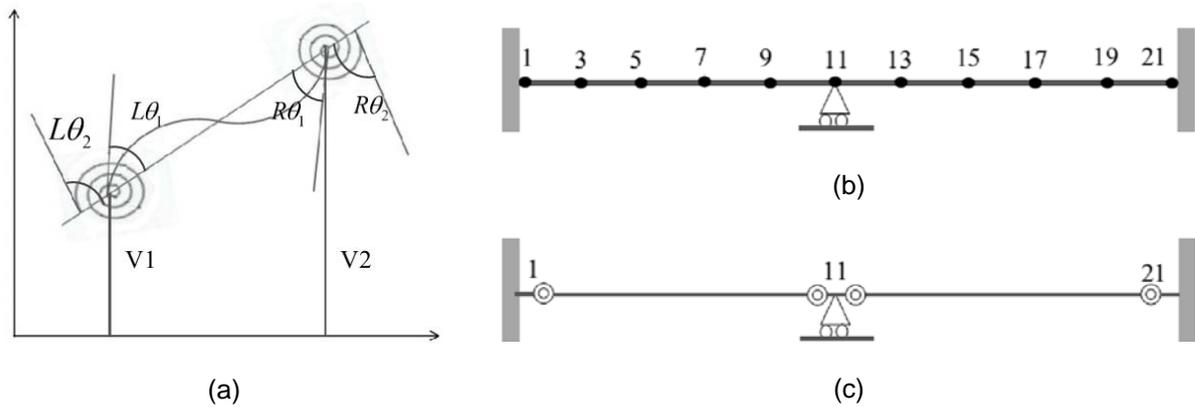
Fig. 1(a) Deformation of an element due to end displacement; (b) two span continuous beam model (make a roller at the intermediate span); (c) representations of joints using rotational springs
