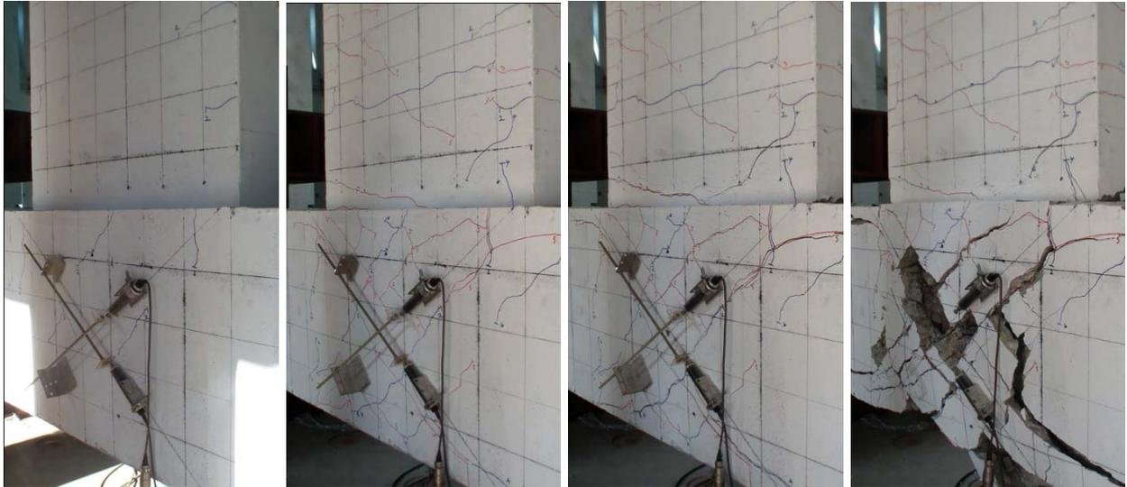
Fig. 8 Observations of RC1 at 0.75%, 2%, 3% and 5% drift ratios
