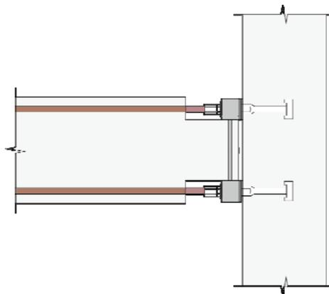
Fig. 1 Pre-tension bolting connection concept
