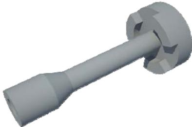
Fig. 3 Embedded nut with anchor rod
