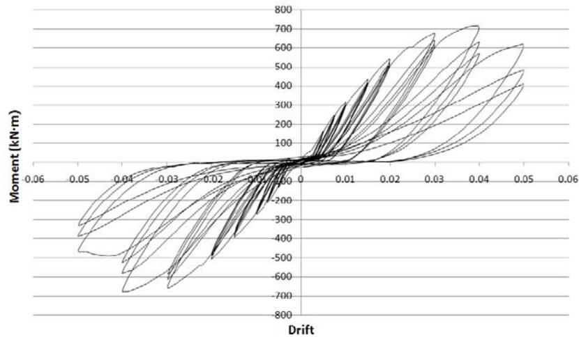
Fig. 6 Beam moment-story drift ratio relationship for PC1
