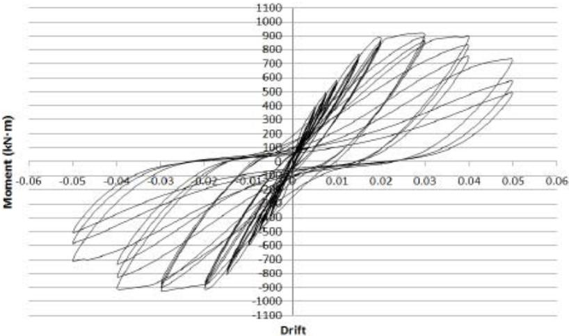
Fig. 5 Beam moment-story drift ratio relationship for RC1
