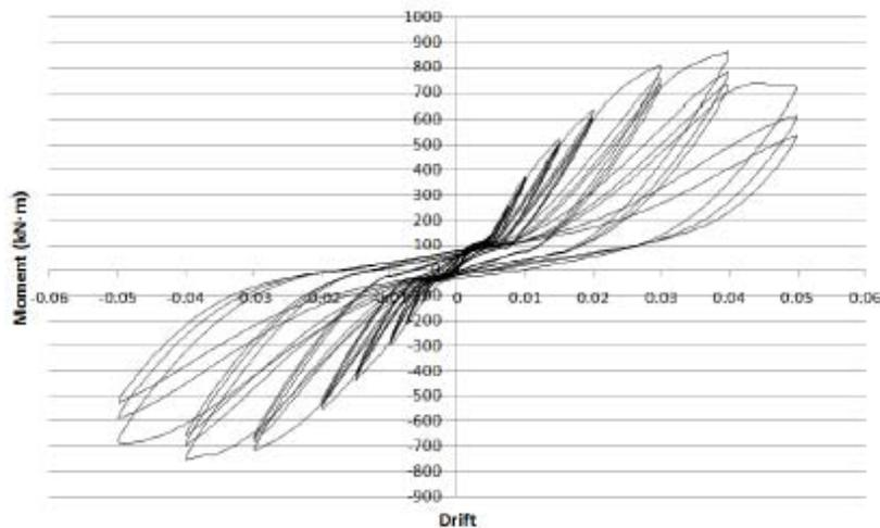
Fig. 7 Beam moment-story drift ratio relationship for PC1-T
