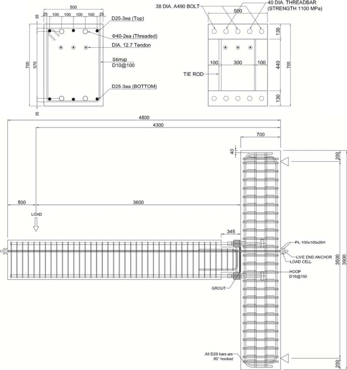
Fig. 4 Specimen drawing (PC2-T)
