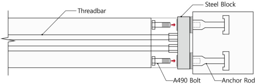
Fig. 2 Pure dry cast method; Beam-to-column connection using pre-tension bolts
