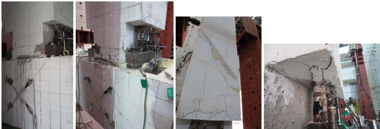
Fig. 10 Observations of PC2-T at 4% drift ratio
