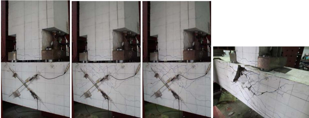
Fig. 9 Observations of PC1 at 0.5%, 2%, 3% and 5% drift ratios
