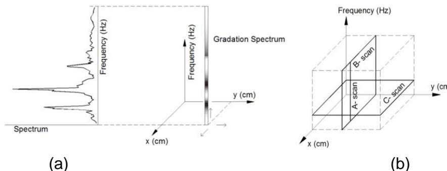
Fig. 2 Illustration of basic principles of 4-D spectrum technique: (a) color/grey scale and position mapping within image volume and (b) layout of image planes within image volume.
