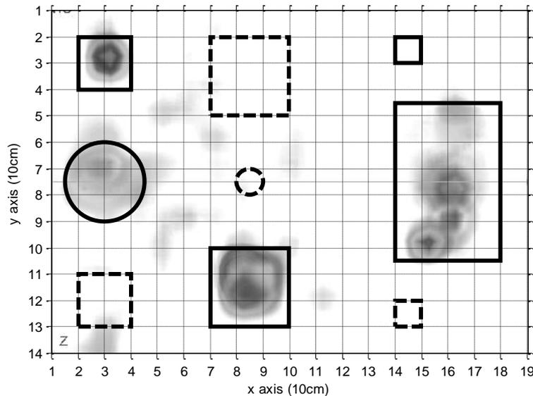
Fig. 6 Top (x-y) perspective of 4-D IE data plot. Data up to 6 kHz collected over entire face of 2.0m×1.5m slab specimen along 10cm square grid
