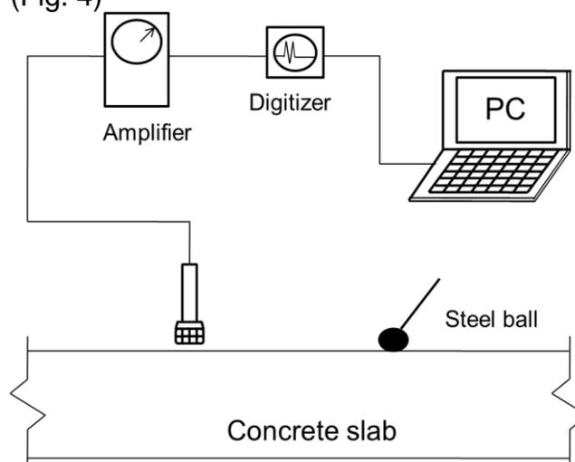
Fig. 4 Experimental test setup for air-coupled impact-resonance test. The air-coupled sensor is positioned as closely on the slab surface.
