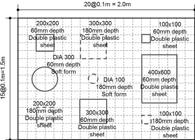
Fig. 5 The 2.0m x 1.5m reinforced concrete slab; The position of near-surface delamination defects are indicated with bold solid lines, those of deep delamination by bold dashed lines. The testing grid is indicated with light dashed lines
