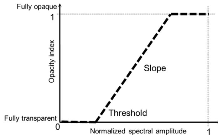
Fig 3. The definitions of the image transparency control parameters.
