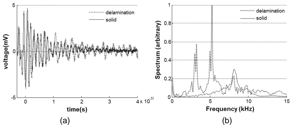
Fig. 1 Impact-echo signal data collected over solid and delamination regions; (a) time-domain and (b) frequency-domain
