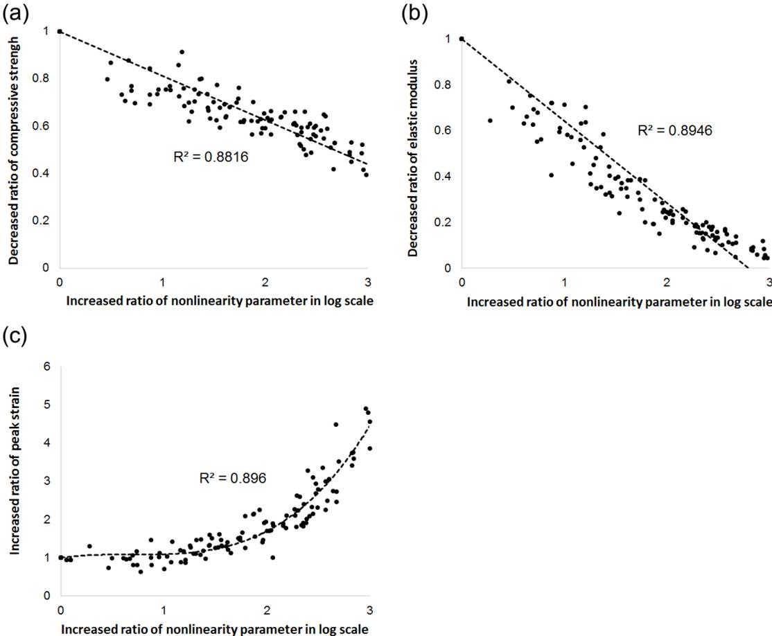
Fig. 1 Relationships between increased ratio of nonlinearity parameter in log scale and: (a) decreased ratio of compressive strength; (b) decreased ratio of elastic modulus; (c) increased ratio of peak strain.
