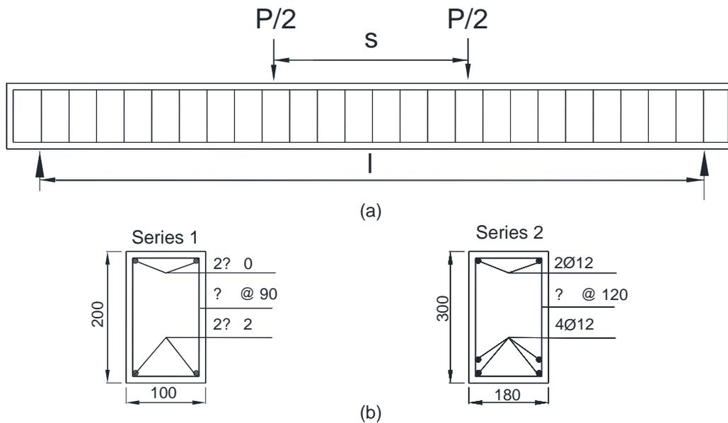
Fig.2: Details of test specimens: (a) elevation (b) section
