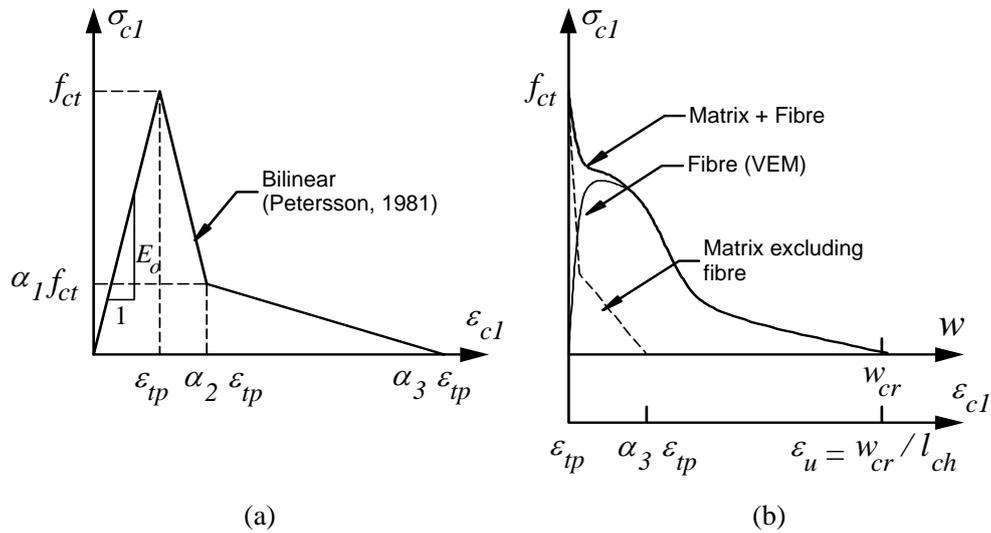
Fig.1: Fibre reinforced concrete in tension: (a) bilinear stress-strain model for concrete matrix (Petersson, 1981) (b) variable engagement model (Voo and Foster, 2009)
