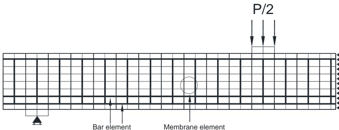
Fig.3: FE mesh for SFRC beams
