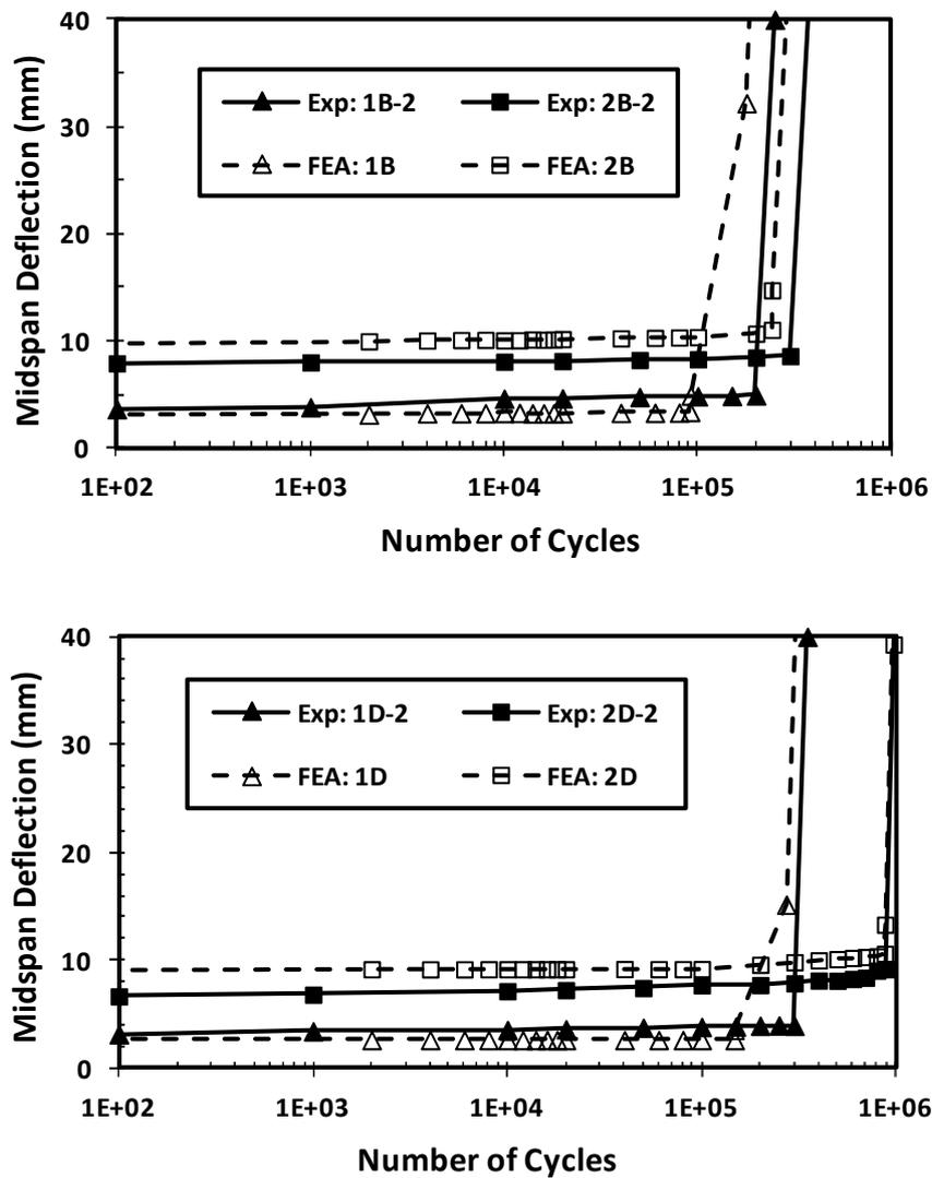
Fig.4- Midspan deflection versus number of cycles at maximum load (a) Beams with 0% fibre (b) Beams with 0.8 % fibres
