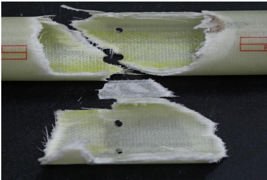
Fig. 6 Fracture shape of pipe specimen(Laminate angle : 30°, ST)
