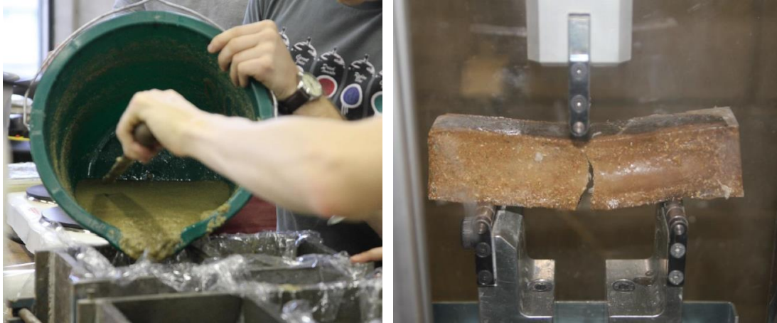
Fig. 2 Material tests by students. Left: sample casting. Right: bending test on Pykrete specimen
