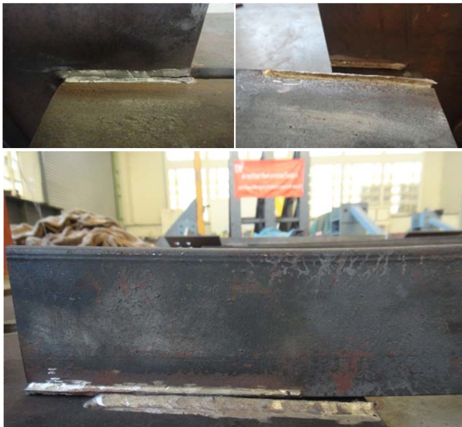
Figure 5 Weld rupture of specimen
