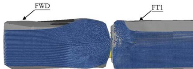
Fig. 27 Behavior of Internal Fluid at the Critical Time(Max. of Equivalent Stress)
