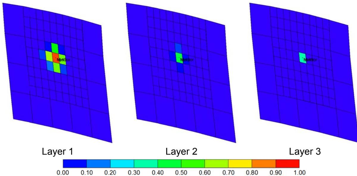
Fig. 16 CO<sub>2</sub> mole fraction of optimum case at soaking time.
