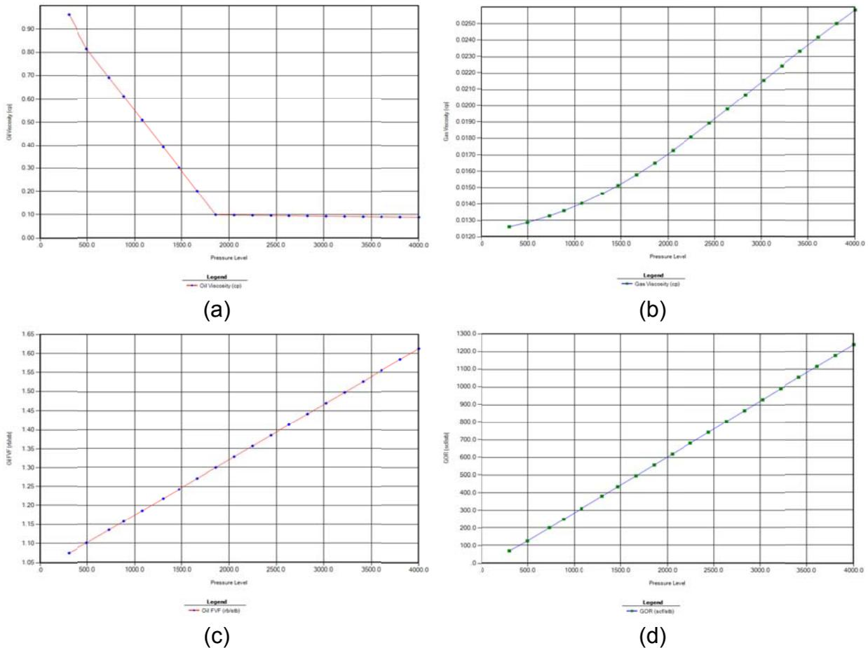
Fig. 2 Experimental data for PVT modelling: (a) oil viscosity, (b) gas viscosity, (c) oil formation volume factor, and (d) gas oil ratio.
