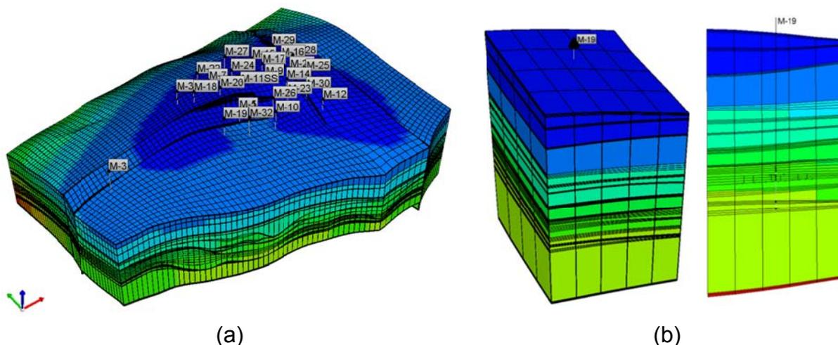
Fig. 1 Reservoir model of M field in Indonesia: (a) full model, and (b) subtracted model.
