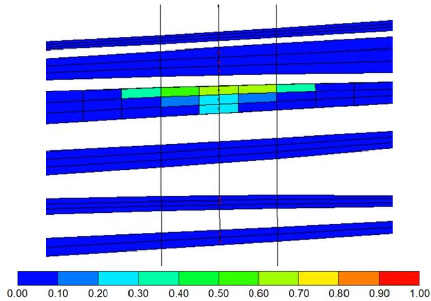
Fig. 11 Gravity overriding effect of injected CO<sub>2</sub>.
