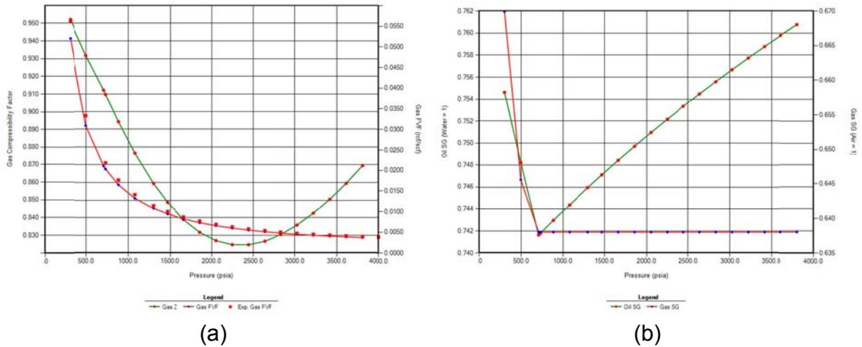
Fig. 4 Results from DL (differential liberation) for PVT modelling: (a) gas compressibility factor and gas formation volume factor, and (b) specific gravities of oil and gas.
