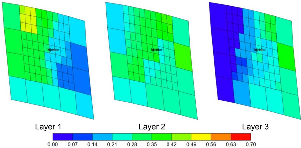
Fig. 14 Oil saturation of optimum case at the end of simulation.
