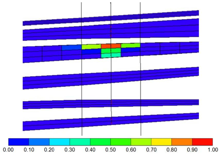
Fig. 17 Gravity overriding effect of injected CO<sub>2</sub> at optimum case.
