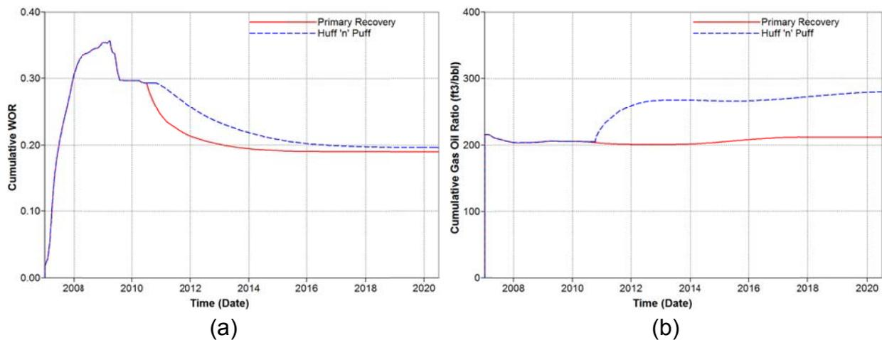
Fig. 9 Cumulative WOR and GOR of primary recovery and Huff and Puff process: (a) cumulative WOR, and (b) cumulative GOR.
