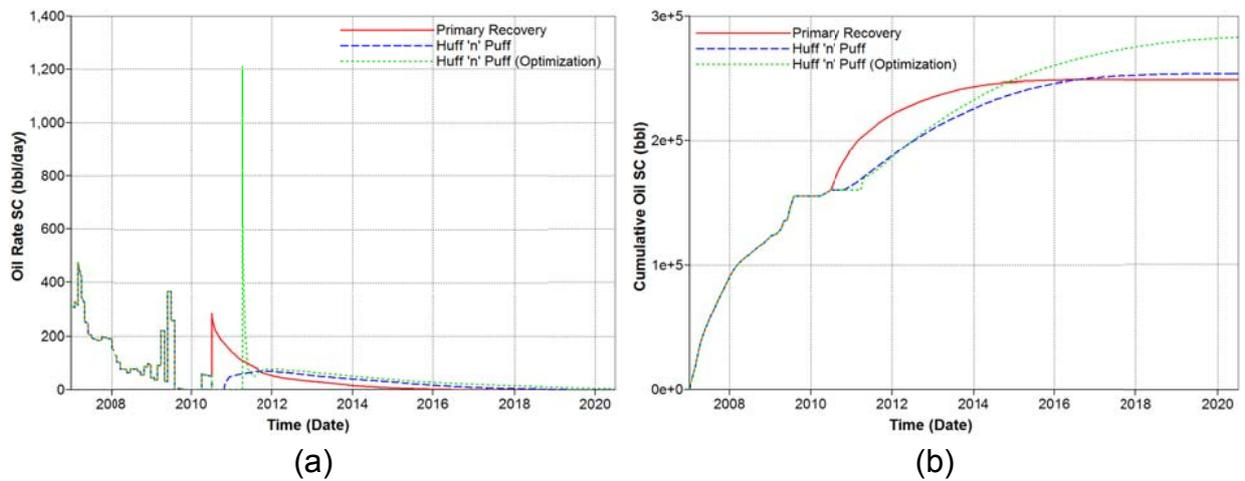
Fig. 13 Oil production of optimized Huff and Puff process: (a) oil rate, and (b) cumulative oil.
