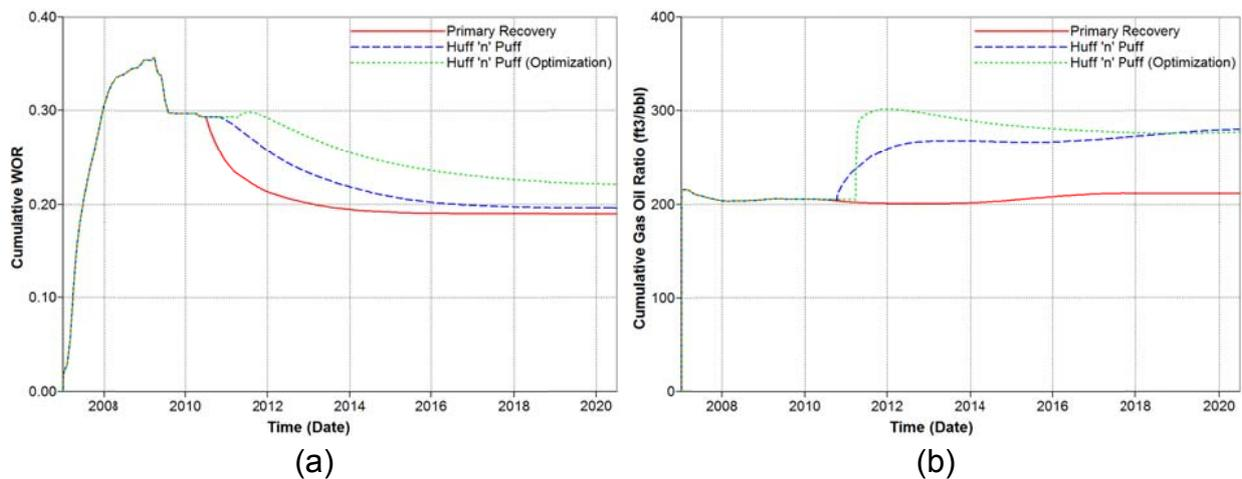
Fig. 15 Cumulative WOR and GOR of optimized Huff and Puff process: (a) cumulative WOR, and (b) cumulative GOR.
