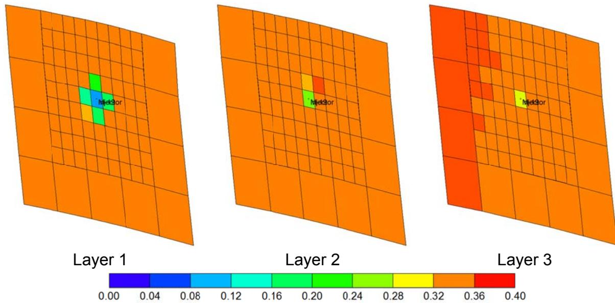
Fig. 19 Viscosity reduction of reservoir oil in optimum case.
