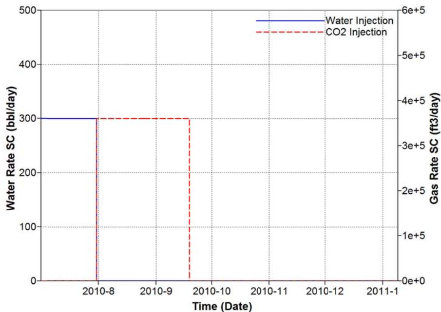
Fig. 6 Schedule for water injection and CO<sub>2</sub> injection.
