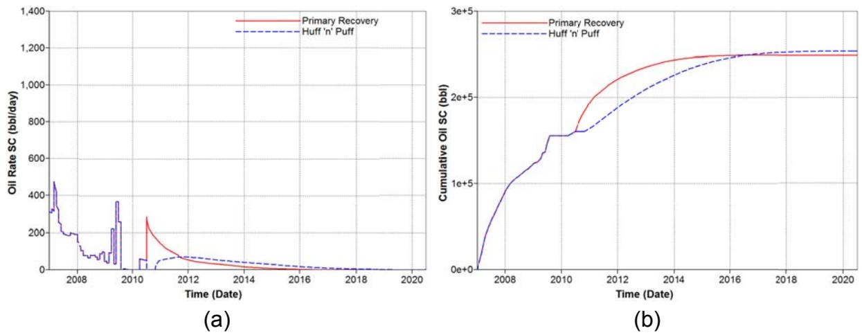
Fig. 7 Oil production for primary recovery and Huff and Puff case: (a) oil rate, and (b) cumulative oil.
