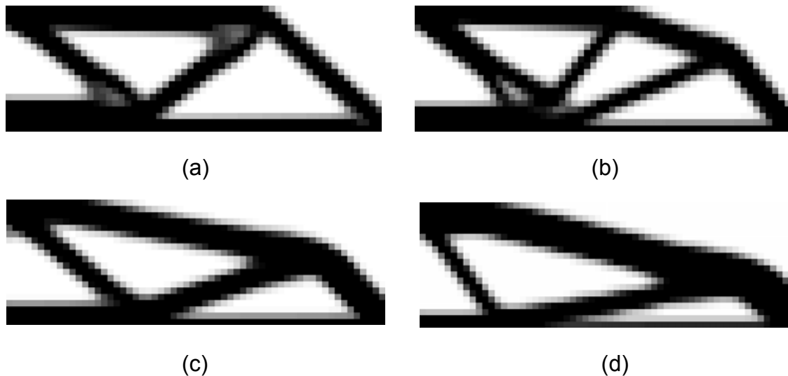
Figure 2. Topology optimization of the orthotropic MBB-beam: (a) isotropic, (b) E_1/E_2 = 4 , (c) E_1/E_2 = 10 , (d) E_1/E_2 = 50 .
