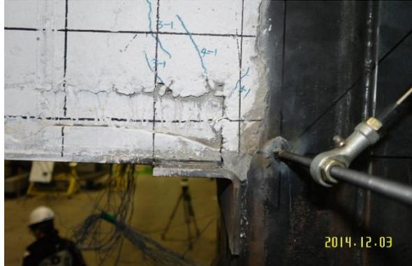
d. CNR bottom : Weld failure
