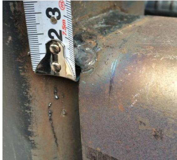
b. CWN-upper groove welded(10mm)
