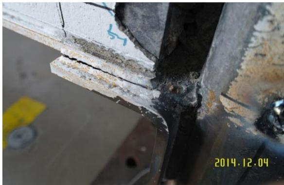
c. CWN bottom plate : Weld failure
