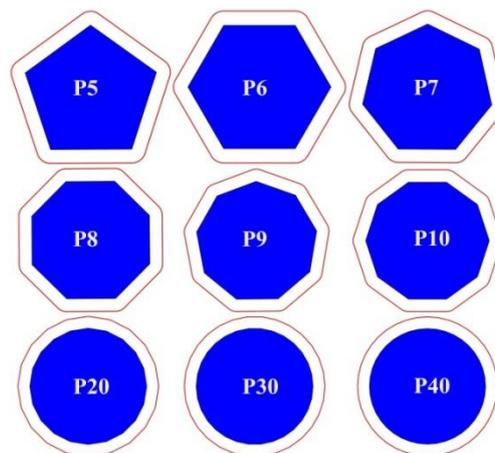
Fig. 4 The construction of ITZ layer around P5~P10, P20, P30 and P40
