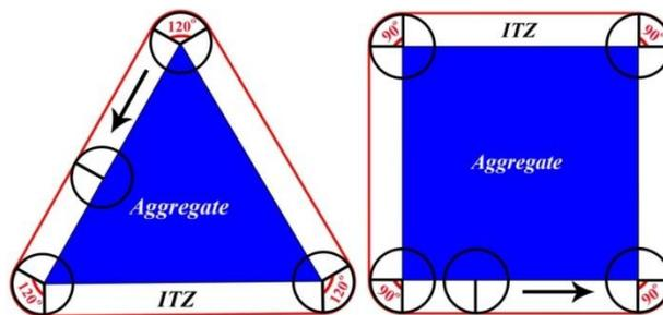
Fig. 2 The construction of ITZ layer around P3 and P4
