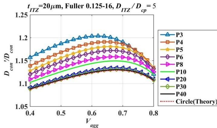
Fig. 11 Influence of polygon shape on the overestimation of concrete diffusivity
