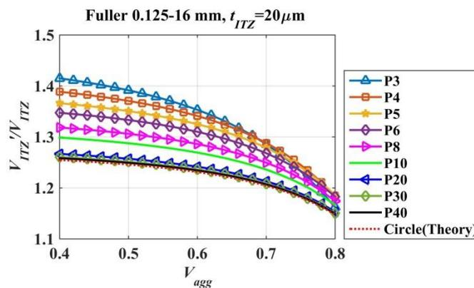
Fig. 10 Effect of polygon shape on the overestimation of ITZ volume fraction
