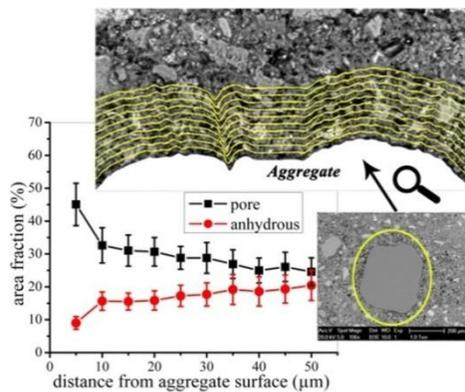
(a) ITZ thickness around aggregate from SEM image, (Gao et al. 2013)
