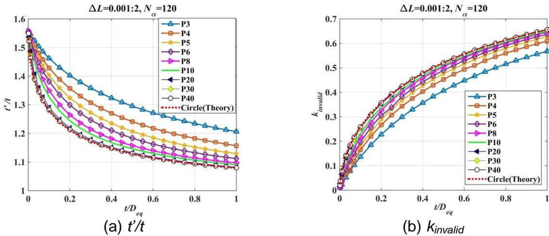
Fig. 8 Effect of actual ITZ thickness  $t/D_{eq}$  on  $t'/t$
