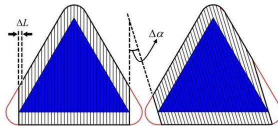
Fig. 5 The planar angle step  $\Delta\alpha$  and spacing  $\Delta L$  between sampling lines
