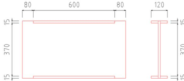
Fig. 14 Detail of embedded H-beam
