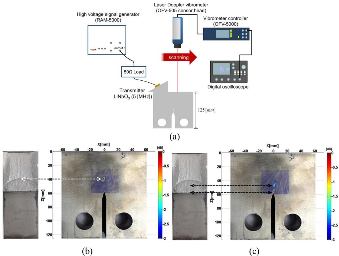
Fig. 2 Measurement system and imaging results, (a) Schematic diagram of experimental apparatus, Cross-section of the specimen with phased array images for (b) Sub-harmonic frequency (2.5 [MHz]) that is assumed to show closed part indicated by white arrow, (c) Fundamental frequency (5 [MHz]) that shows open part indicated by black arrows.
