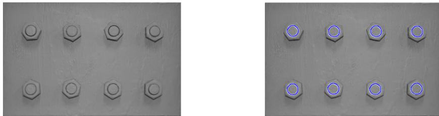
(a) Corrected image for distortion                      (b) circles found by circular Hough transform
