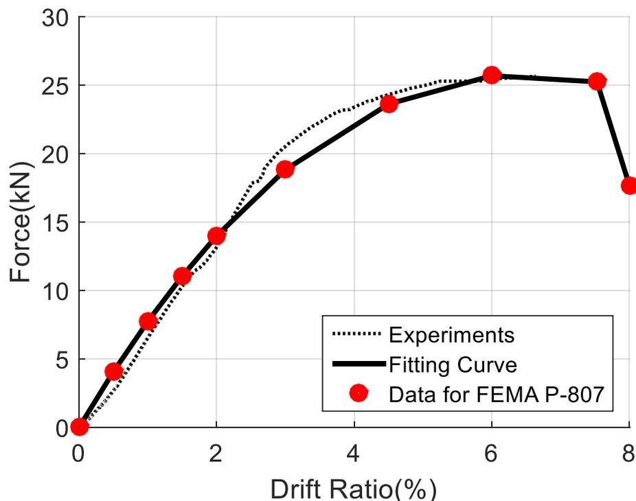
Figure 4. Testing data and numerical model of CLT
