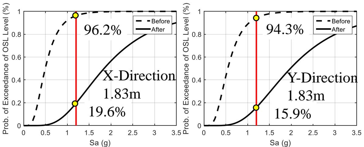
Figure 9: Fragility curves for each direction of the example building with 1.2g, 20% POE.
