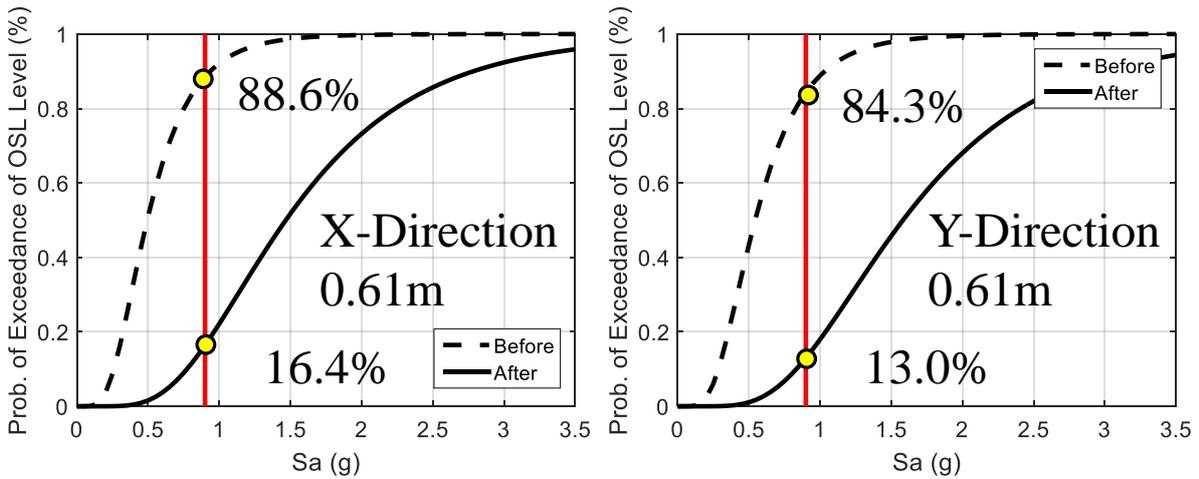
Figure 8: Fragility curves for the x- and y-direction of the three-story example building.
