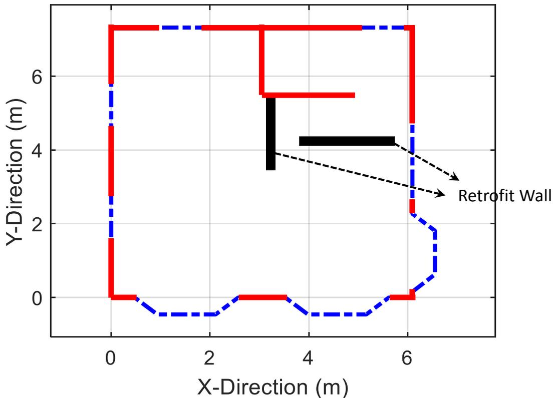
Figure 10: Retrofit Design for the example building with 1.2g, 20% POE.
