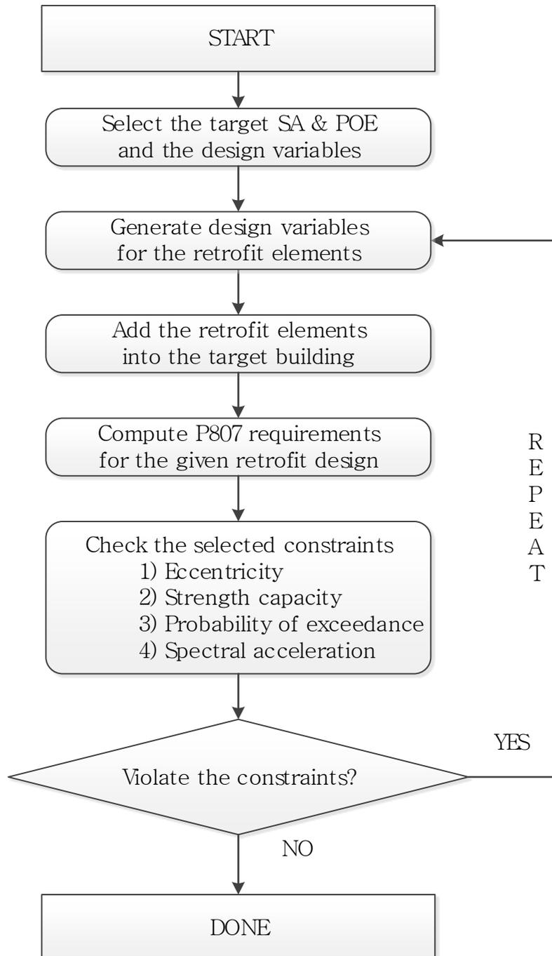
Figure 1: Overall procedure of the FEMA P-807 guidelines (Park and van de Lindt, 2014).
