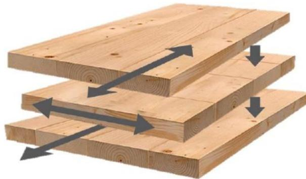
Figure 3. Schematic overview of CLT layer configuration (Laguarda Mallo and Espinoza, 2014)
