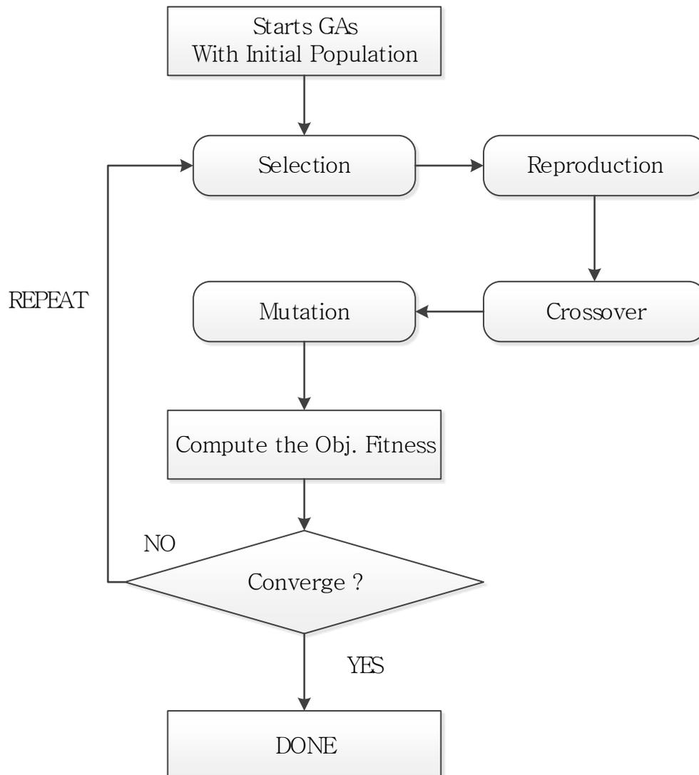
Figure 2. Schematic procedure for GAs.
