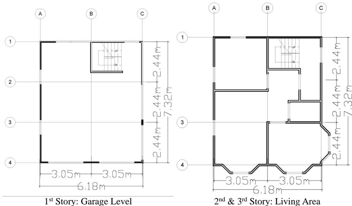
Figure 5: Floor plan for the three-story residential structure with first story parking garage (van de Lindt et al., 2013).
