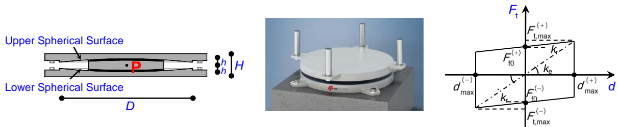
Fig. 9 Cross section, view and schematic response cycle of a DCSS isolator with equal sliding surfaces
