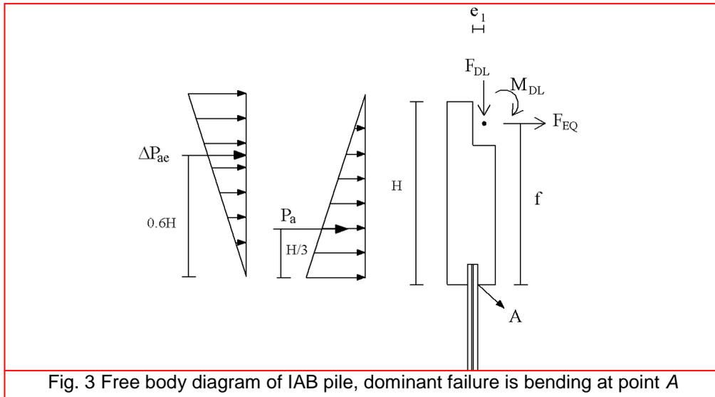
Fig. 3 Free body diagram of IAB pile, dominant failure is bending at point A
