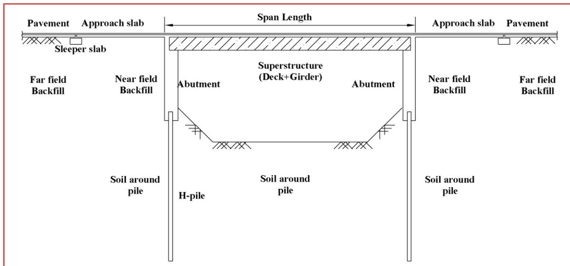
Fig. 2 Longitudinal section of the IAB
