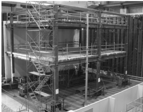
Fig. 9 Three storey two bay steel frame (Nakashima 2006)
