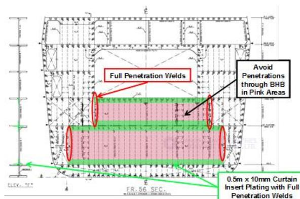
Fig. 1 Typical BHB curtain design shipboard installation (Cowardin et al. 2013)
