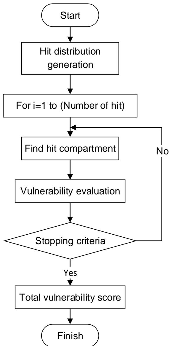
Fig. 1 Vulnerability evaluation algorithm
