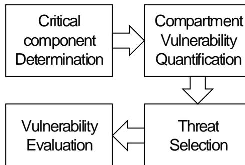
Fig. 2 A simplified vulnerability evaluation flowchart
