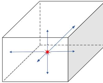
Fig. 4 Internal blast pressure in the compartment
