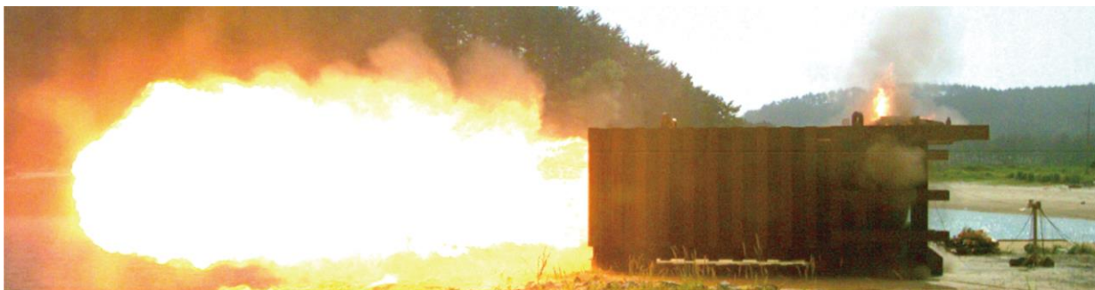
Fig. 3 Chamber model internal blast test
