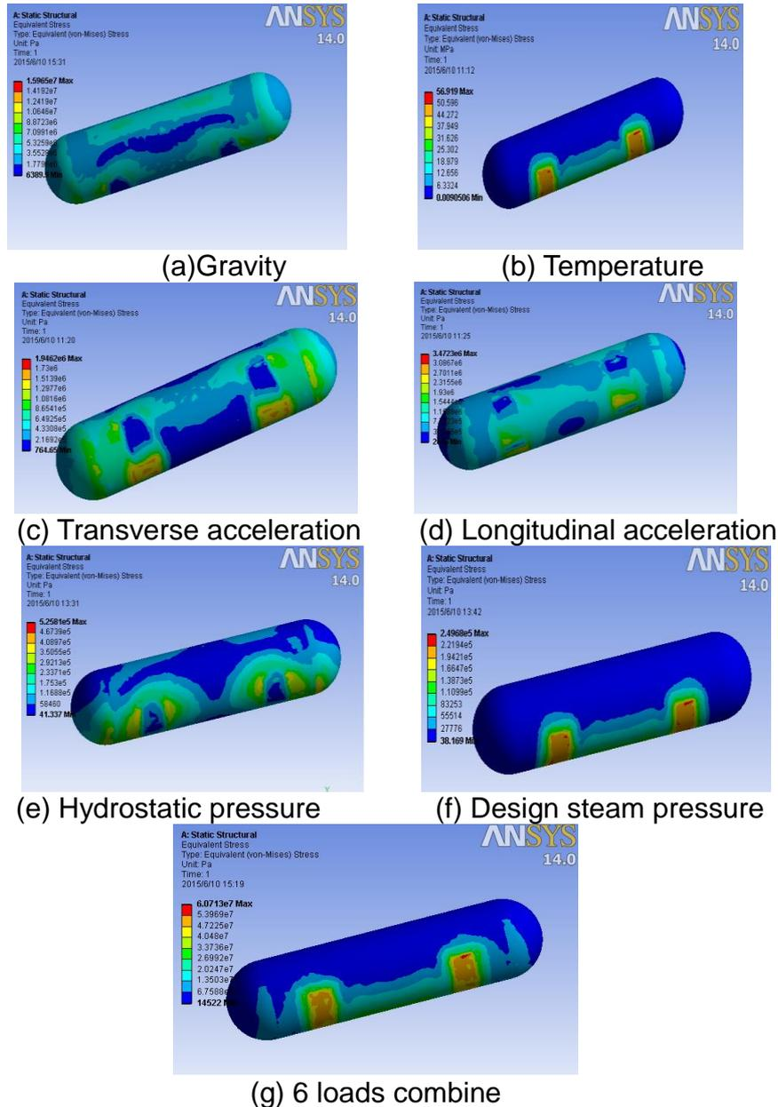
Fig. 6 Stress analysis of tank under different loads
