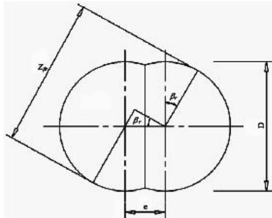
Fig. 2 Liquid height on transverse plane
