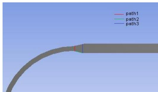
Fig. 7 Joint between cylinder and head
