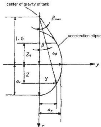
Fig. 1 resultant acceleration ellipse on Y-Z plane
