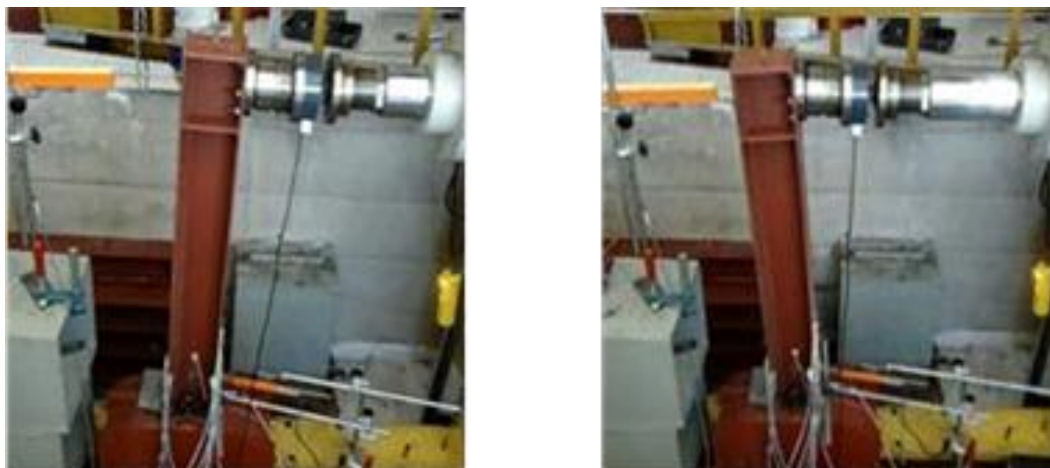
Figure 7. Application of a cyclic lateral displacement at the pile top (a) push, (b) pull direction.
