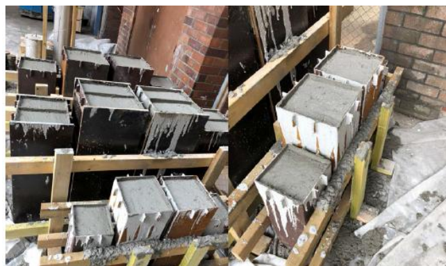
Fig. 4 High strength steel slenderness tests, (Huang et al, 2019)
