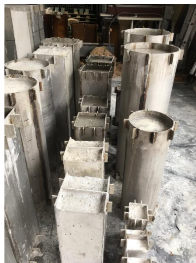
Fig. 6 Stainless steel slenderness tests, (Kazemzadeh Azad, Li and Uy, 2019)
