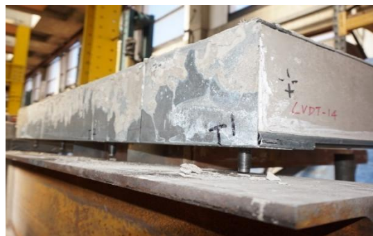
Fig. 15 Studs at the other shear span (no fracture during testing and dismantling; B1b)
