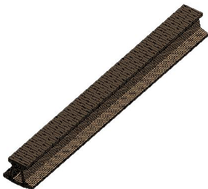
Fig. 2. Finite Element Model of High-Speed Maglev Track Beam
